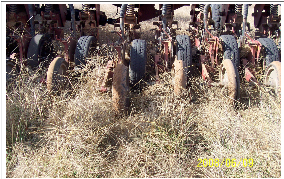
Fig. 3. Modern machinery is well suited to sowing annual grain crops into perennial groundcover, a technique known as 'pasture cropping'
