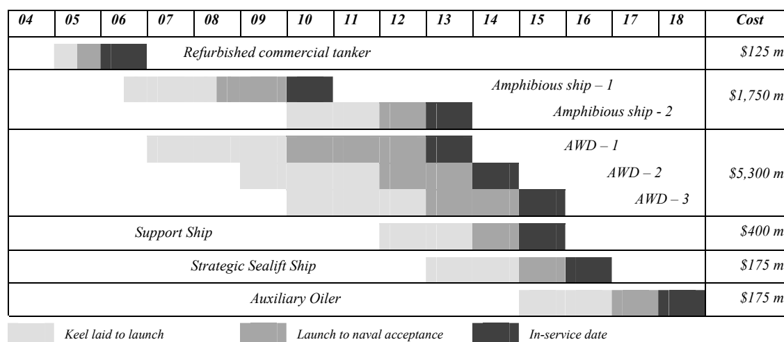
Figure 1 Indicative naval construction schedule 2004 – 2018 (Source: Mark Thomson 56 )
