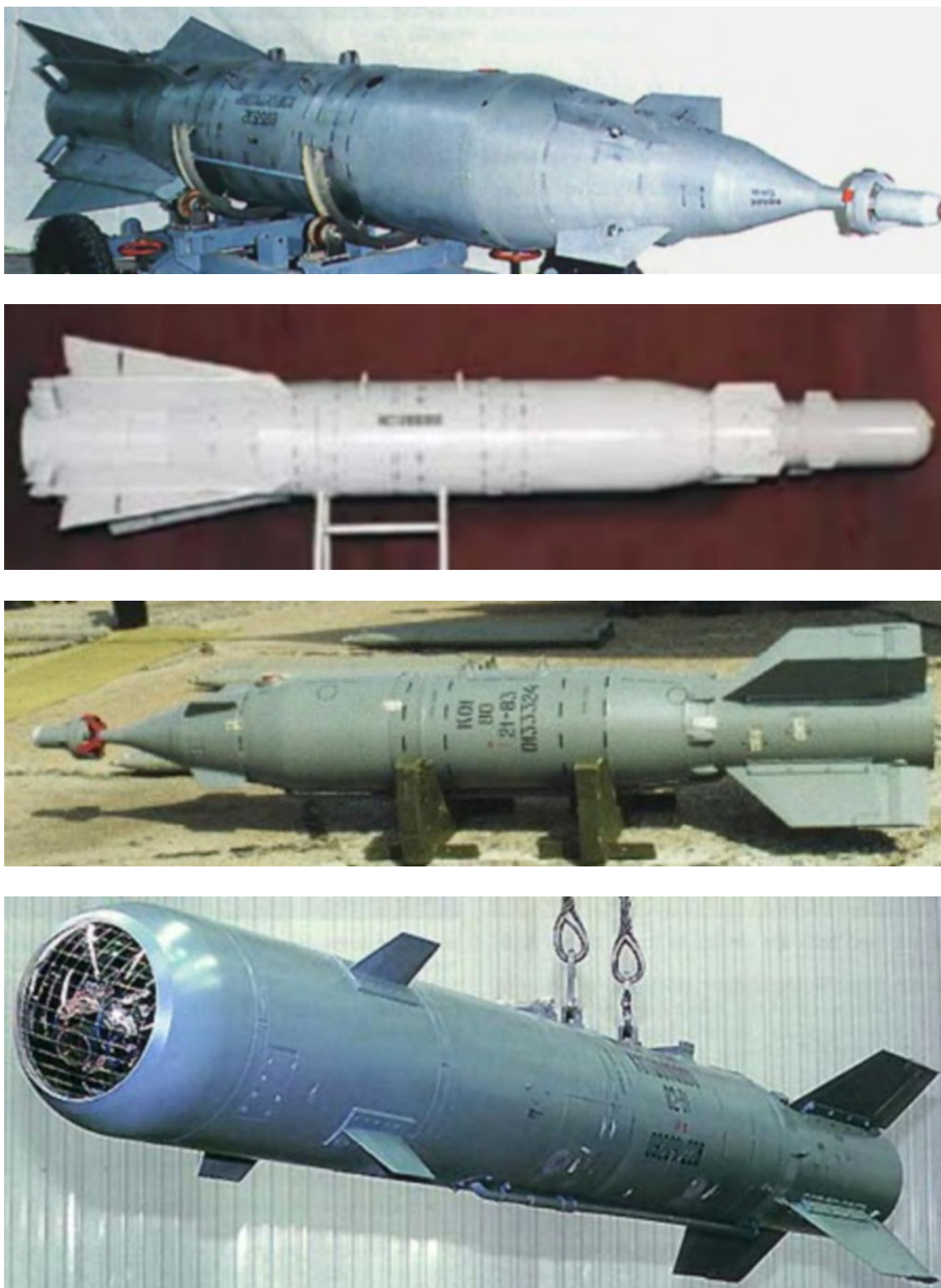
Figure 40: Russia is actively marketing smart bombs for the Sukhoi fleets supplied to the PLA. These images depict the laser and television guided KAB-1500 (1500 kg) series and KAB-500 (500 kg) series guided bombs, available in bunker busting and standard explosive variants. These weapons are broadly equivalent to the US Raytheon GBU-10, GBU-24 carried by RAAF F-111s, and the Boeing GBU-15 which was carried by the F-111 during the 1980s (Rosvooruzheniye).
