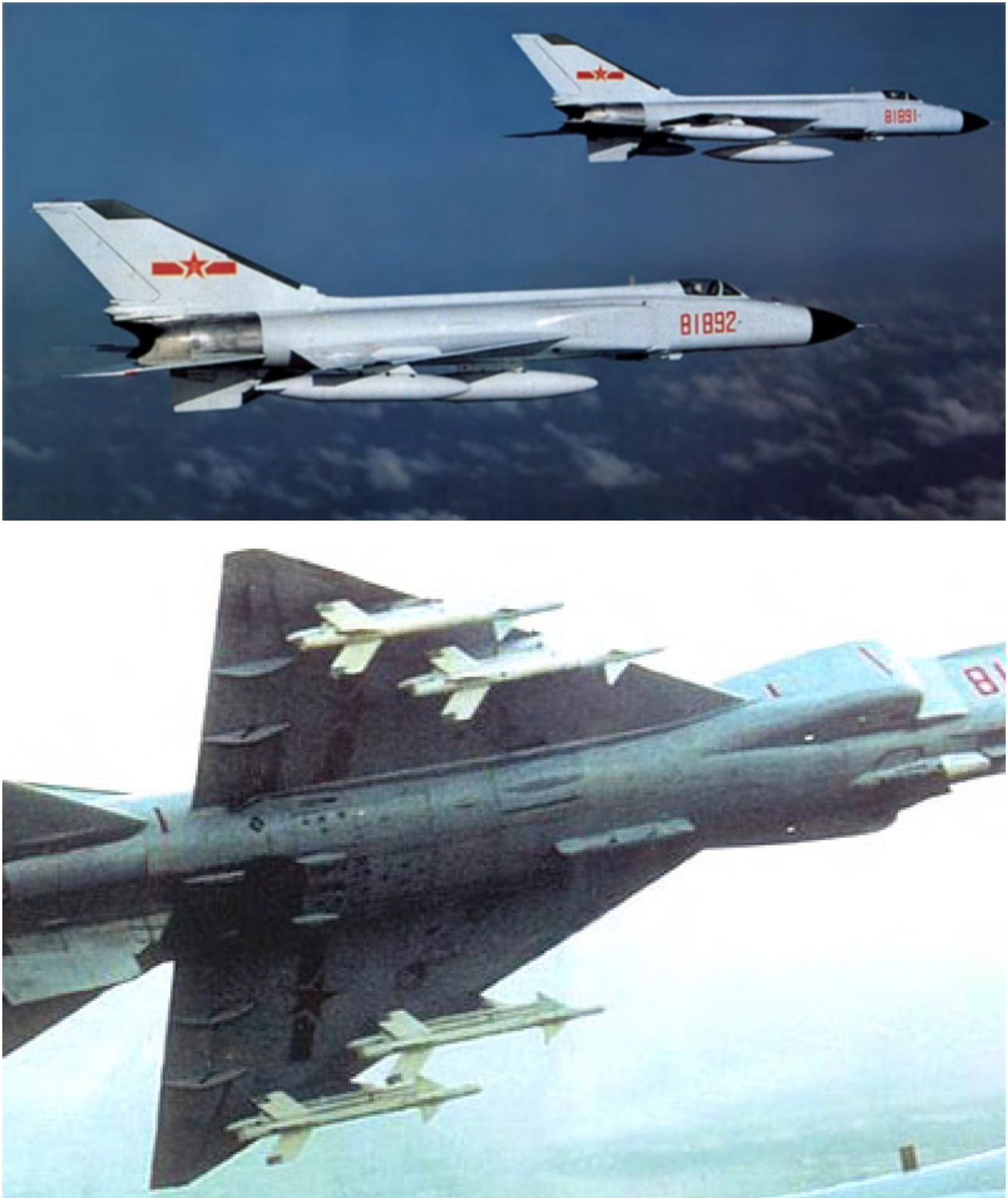
Figure 22: The J-8-II Finback B is an indigenous Chinese multirole fighter and is broadly equivalent to the Russian Su-15/21 series and RAF Tornado ADV/IDS. The lower image depicts a J-8-II armed with PL-8 missiles, reversed engineered from the Israeli Python 3 (PLA).
