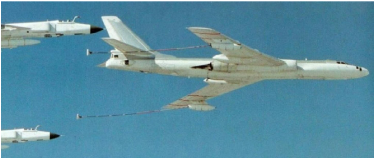
Figure 20: The Xian H-6 is the basis of China's indigenous aerial refuelling tanker program. Development was reported to be initially a collaboration with Flight Refuelling Limited in the UK during the 1980s. With the questionable usefulness of the Badger as a conventional strike aircraft, it is likely many more will be converted to tankers, especially given the low age of much of the Badger fleet. As a tanker the Badger compares closely to the now retired RAF Victor K.2 (PLA).
