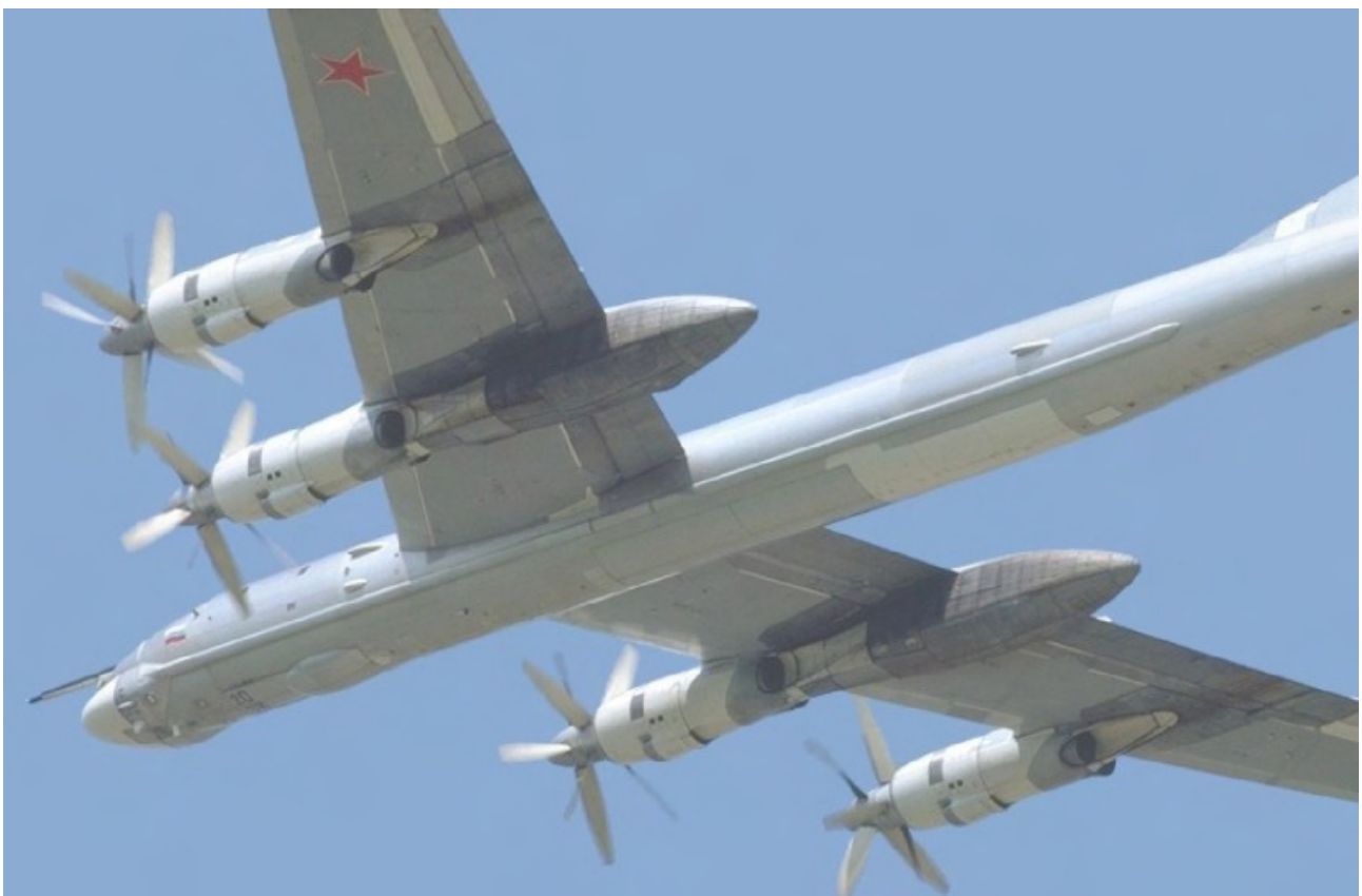
Figure 11: The Tu-95MS Bear H cruise missile carrier has been publicly offered to the PLA by Russia. A direct equivalent to the US B-52H, these long range aircraft remained in production until 1993, making the Russian fleet 'young' in accrued airframe hours (US DoD/RuAF).
