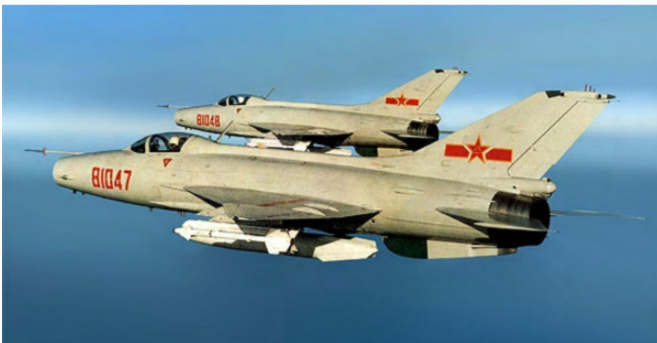
Figure 21: China continues to manufacture and operate a range of legacy types. The Q-5 is an indigenous evolution of the Russian MiG-19 Farmer and is broadly equivalent to the A-4 Skyhawk. Around 600 are in service. The J-7 is an indigenous evolution of the Russian MiG-21 Fishbed and is broadly equivalent to the Northrop F-5 series, but faster and more agile. Around 700 are in service (PLA).
