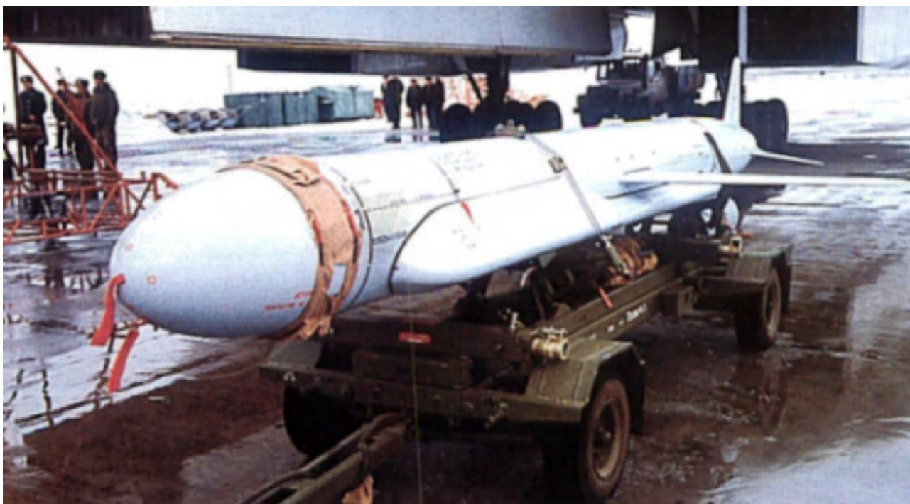
Figure 32: The Raduga Kh-55 Granat or 'Tomahawk-ski' (AS-15 Kent) cruise missile was developed as an equivalent to the US AGM-86 carried by the B-52H and the US RGM-109 Tomahawk carried by submarines, and arms the Tu-95MS and Tu-160 strategic bombers. Numerous reports claim the PLA illegally acquired Kh-55 rounds from the Ukraine five years ago, and legally purchased tooling for the non-nuclear Kh-65 variant of this missile. The lower image shows the improved Kh-55SM with conformal fuel tanks, providing a range of up to 1,600 nautical miles (RuMoD).
