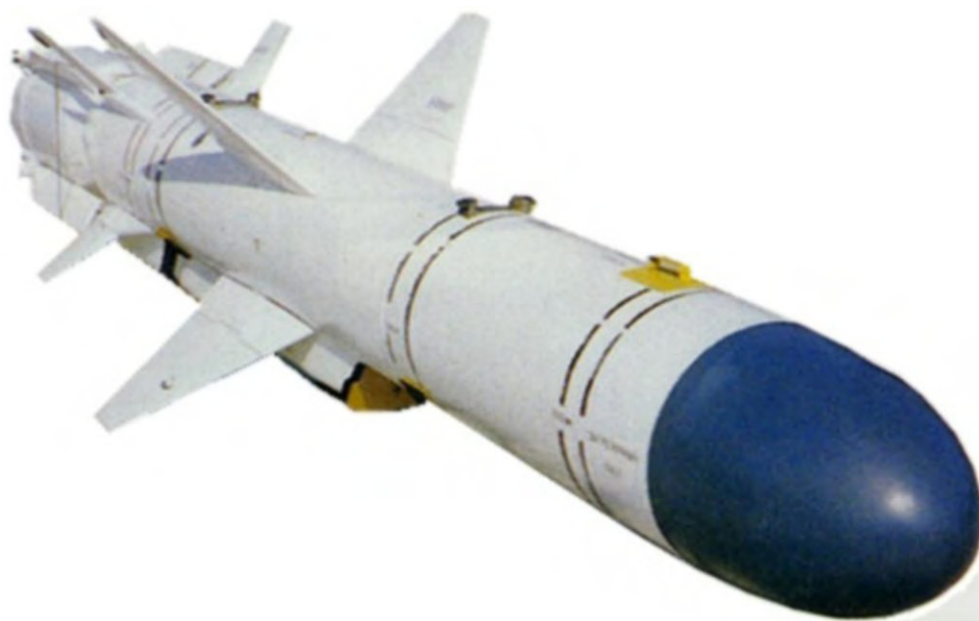
Figure 39: The Kh-59M/D series stand-off weapon is a direct equivalent to the AGM-142 missile now being integrated on the RAAF's F-111C, and carried by the US B-52H (Upper). Evolved from an anti-radar missile, it is now available with an optical seeker. The PLA-N is reported to have ordered an anti-ship variant equipped with a radar seeker, designated the Kh-59MK2 (-). Dubbed the 'Kharpunski' the Kh-35U Uran is the Russian equivalent to the US RGM-84/AGM-84 Harpoon carried by the F-111C and RAN warships (Lower). The missile is available in surface launched and air launched versions (Rosvooruzheniye).
