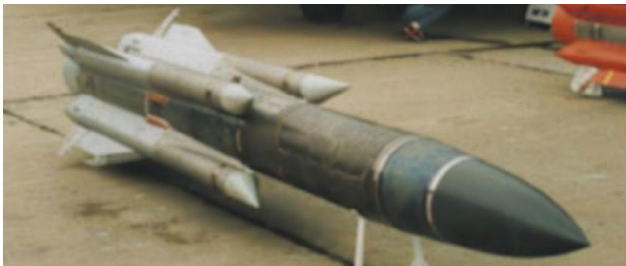
Figure 38: The supersonic ramjet Kh-31P was originally designed as an anti-radar missile to suppress NATO air defences. Since the end of the Cold War it has evolved an extended range variant, the Kh-31MP, and an anti-ship variant equipped with a radar seeker, the Kh-31A/MA. It has no equivalent in the Western inventory. The PLA is reported to have licenced this weapon (RuMoD).
