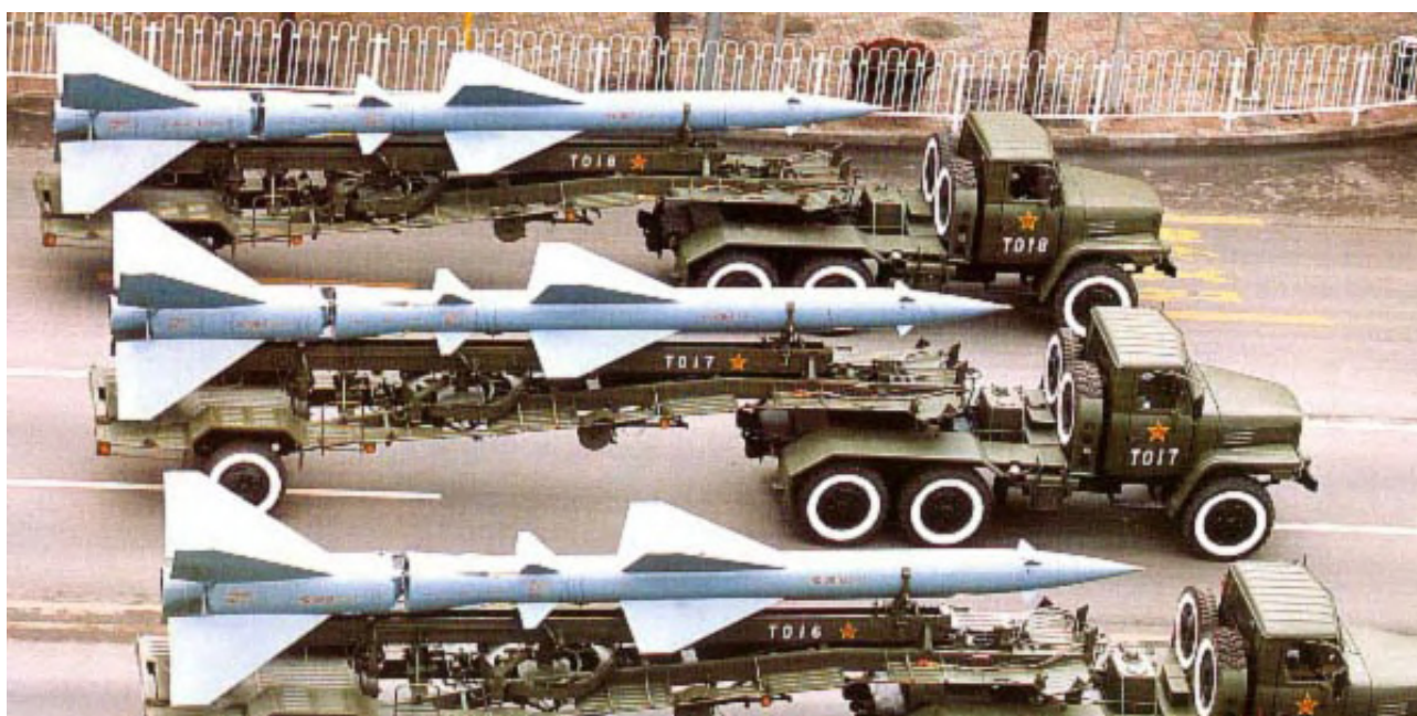
Figure 29: The PLA continues to operate variants of the legacy HQ-2 (SA-2 Guideline) series strategic SAM system. Unlike the semi-mobile Soviet original, the PLA employs a large number of fully mobile HQ-2 Transporter Erector Launchers making this variant significantly more survivable against defence suppression aircraft (PLA).
