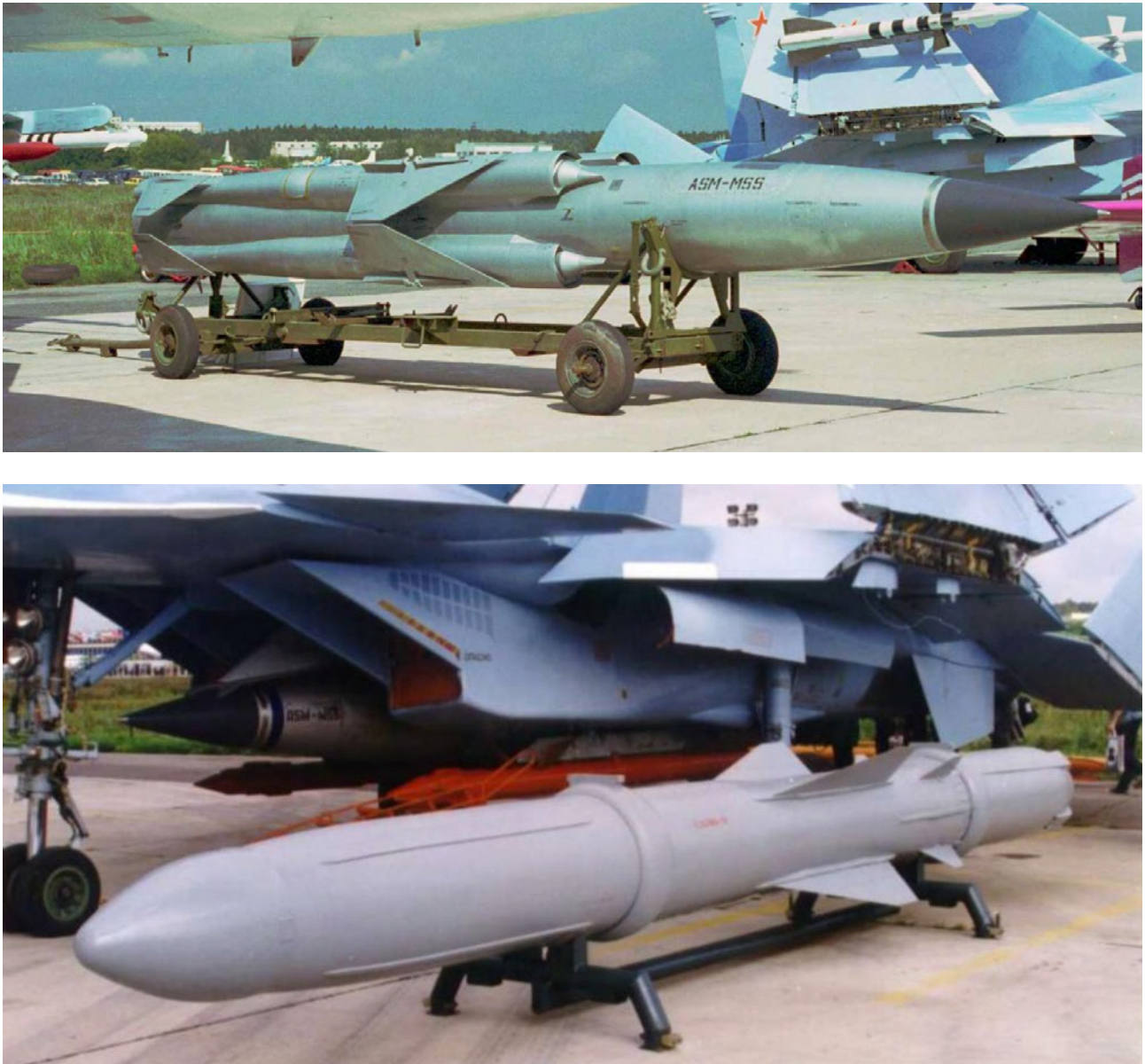
Figure 34: Raduga Kh-41/3M-80/3M-82 Moskit (Upper). This supersonic sea skimming anti-ship cruise missile has been exported to the PLA in its ship-launched variant. The missile is on offer as the air launched Kh-41 for the Su-30MK fighter. There is no Western equivalent to the Moskit (Rosvooruzheniye). OKB-52 3K-55/3M-55 Yakhont (Lower). This supersonic sea skimming anti-ship cruise missile has been licenced to India for domestic manufacture. It has been reported as the armament for latter 956E series destroyers to be supplied to the PLA-N. There is no Western equivalent to the Yakhont/Brahmos (Rosvooruzheniye/NIC).
