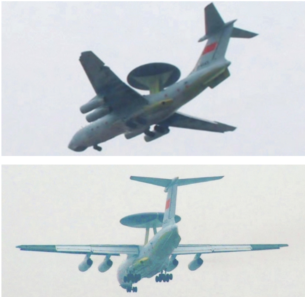
Figure 9: China was reported to have ordered several examples of the Russian A-50E AWACS in the wake of the aborted deal to source the better Israeli A-50I Phalcon variant. Since then photographs have emerged of an indigenous conversion, based in concept on the Israeli A-50I. The images illustrate the use of a phased array radar, similar in technology to the new RAAF Wedgetail - the A-50I radar offered by Israel to China was a variant of the radar offered to Australia for the AIR 5077 bid (via Internet).
