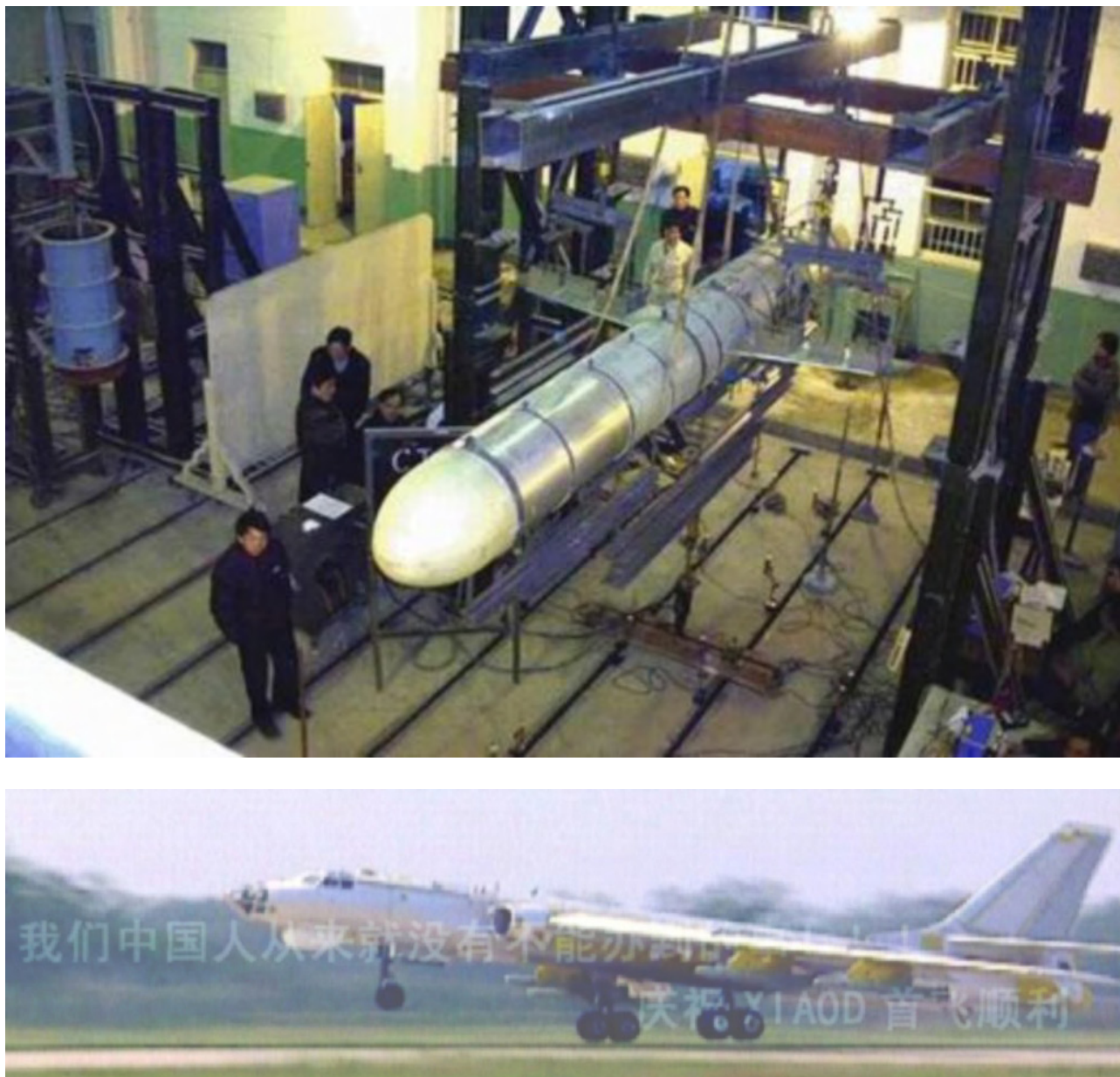
Figure 33: The PLA has had a long running program aimed at developing indigenous long range cruise missiles for submarine and air launched applications. The upper image depicts a submarine launched cruise missile very similar to the US RGM-109 Tomahawk, believed to be of the HN-1/HN-2/HN-3 series, the lower image a H-6M Badger prototype carrying four missile shapes resembling the Kh-55/65 series (PLA).
