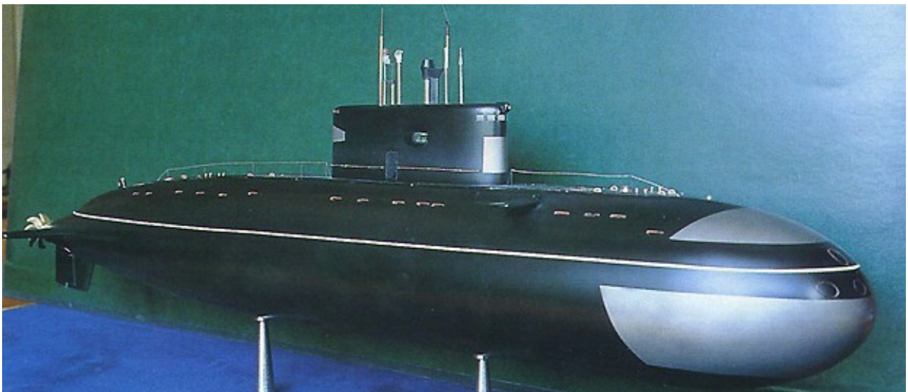
Figure 26: The PLA acquired a pair of Project 877EKM Kilo diesel-electric submarines, followed by a pair of enlarged Project 636 Kilo boats, armed with the 3M-54 series cruise missile. More recently another eight Project 636 Kilo boats were ordered. These low signature boats are considered difficult to defeat (Rosvooruzheniye).
