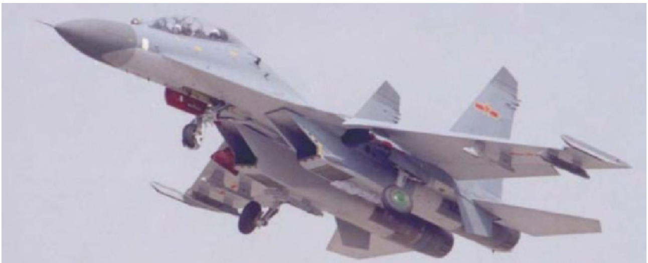
Figure 4: The KNAAPO/Shenyang J-11 is an imported or licence built Russian Su-27SK/UBK long range multirole fighter, broadly equivalent to the US F-15C Eagle. Licence production was recently suspended while negotiations continue for the latter 100 Chinese built models to be delivered in a later configuration, likely the Su-27SMK with precision weapons capabilities. Direct imported Su-27SK/UBK numbers are usually cited at 76 aircraft to date. It is not known whether the Saturn AL-41F supersonic cruise engine is being discussed for the second tranche J-11 build, the AL-41F having entered production last year. Current planning sees around 300 Su-27/J-11 in service by 2015 (PLA).
