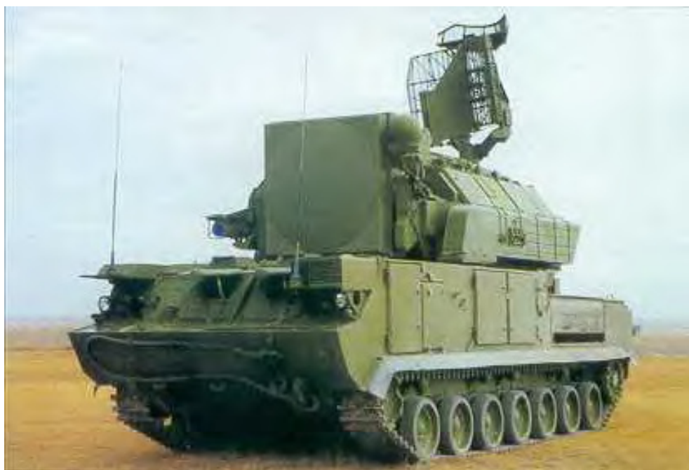
Figure 31: The PLA acquired several batteries of the Tor M1 (SA-15 Gauntlet) point defence SAM during the 1990s. With phased array capability, this system is difficult to jam (Rosoboronexport).
