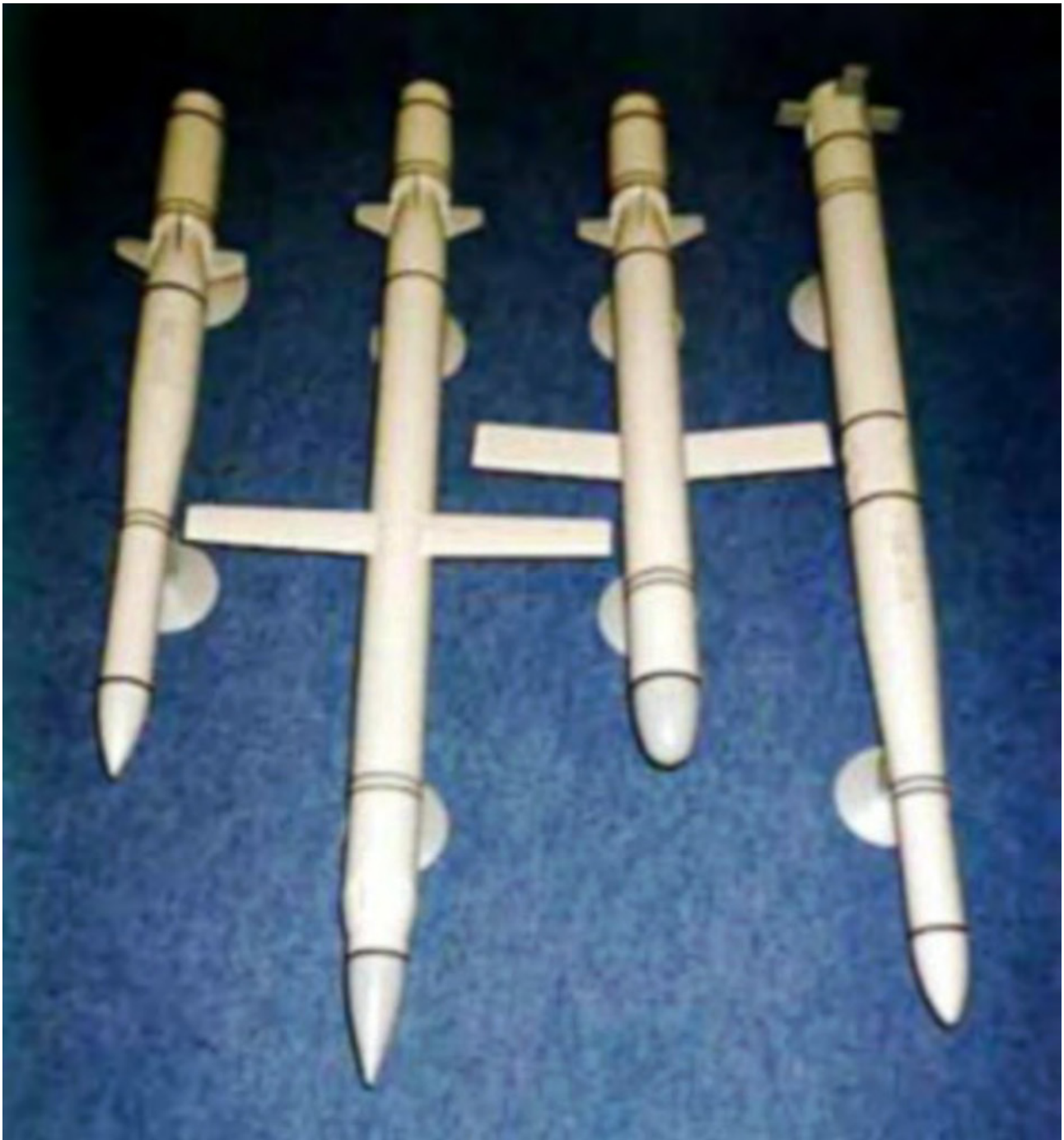
Figure 35: Novator 3M-54 Alfa/Club. This family of subsonic and supersonic sea skimming anti-ship cruise missiles has been exported to the PLA. The Club suite includes the subsonic 3M-54E1 anti-ship and 3M-14E land attack missiles which resemble a shortened Tomahawk, and the supersonic 3M-54E anti-ship missile. The Club is available in ship-launch, submarine-launch and air-launch variants, the submarine-launch variant is now in service. The land attack 3M-14E recently entered production. There is no direct Western equivalent to the 3M-54E (Rosvooruzheniye/NIC).
