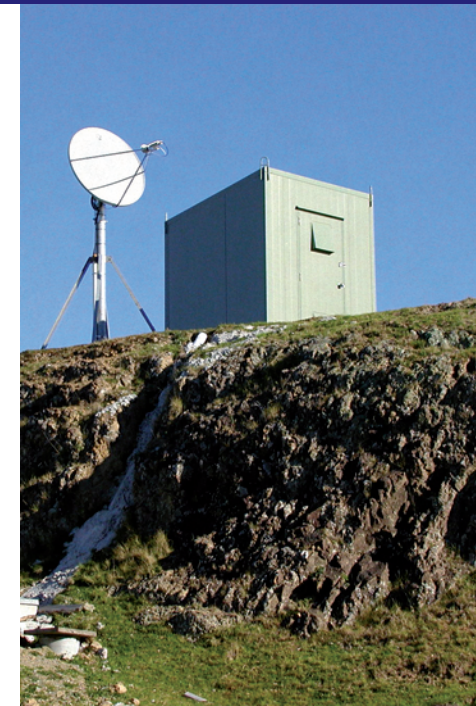
▲ GeoNet provides continuous monitoring of seismic activity throughout New Zealand. This site at Puketiti, south of Te Puia Springs near Gisborne city, has been operational since 1989, and was upgraded by GeoNet with satellite telemetry in 2003.
