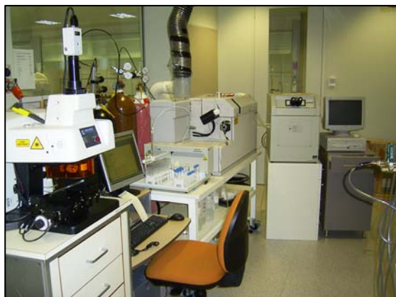
Figure 5: The New Wave 213nm laser system and Agilent ICP-MS instrument at UWA (2006)
