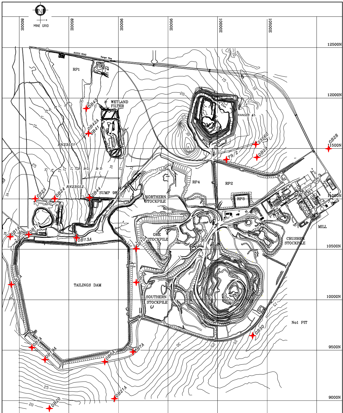
Figure 6 – Groundwater monitoring (ERA) of the Ranger Project (ERA-RAER, 2001)
