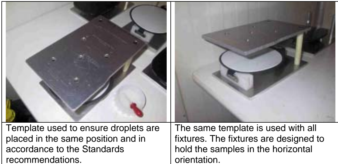
Figure 8.17 Vehicle Fuel Filler Door Test Fixtures
