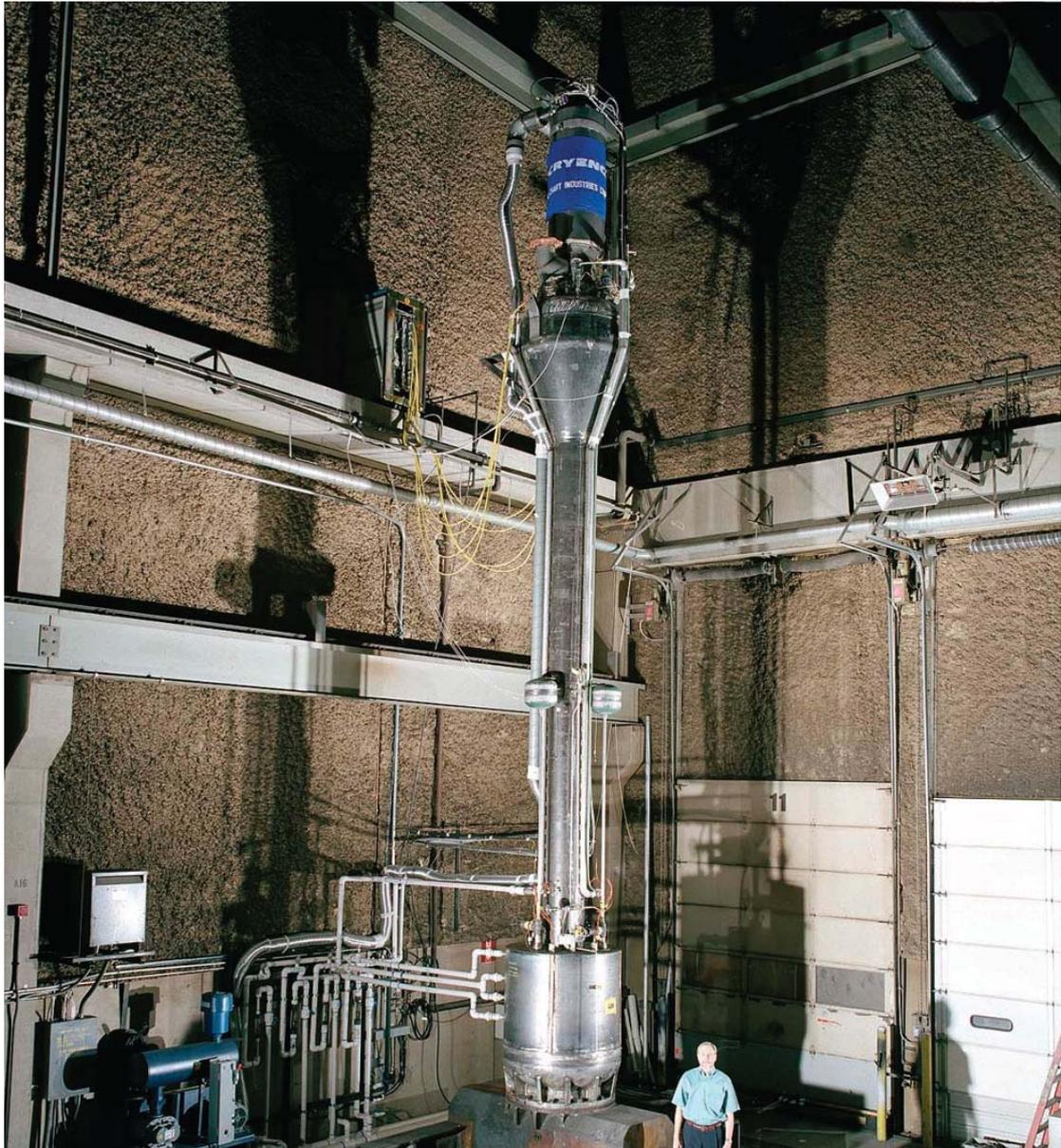
Prototype 500 GPD Natural Gas Acoustic Liquefier (minus 165 degrees C) Produced by Chart at Denver, Colorado, USA.
