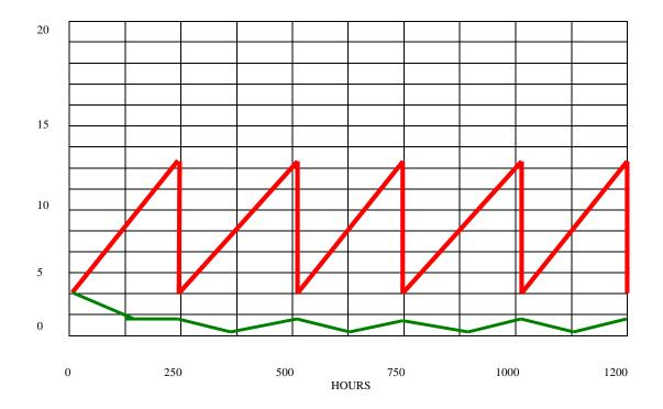
Regular 250hr oil drain interval level of cleanliness
