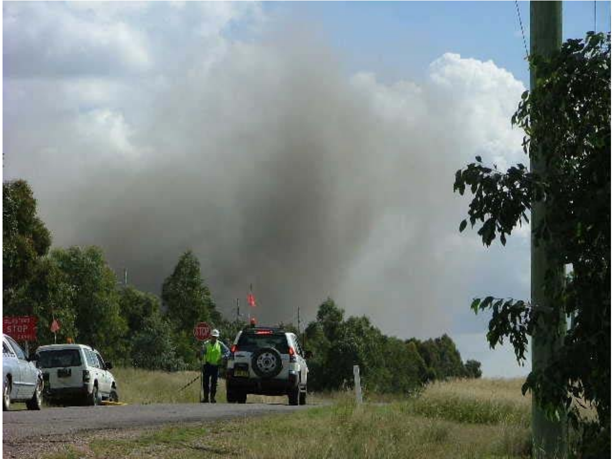
Figure 3: Dust cloud from blasting overburden at Bengalla Mine. Cloud drifting N/W over public road "Wybong Road" and towards occupied residences less than 200 meters away to the right of photo.
