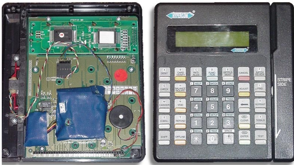
Modified POS skimmer (Japan). Captures data internally for later retrieval
