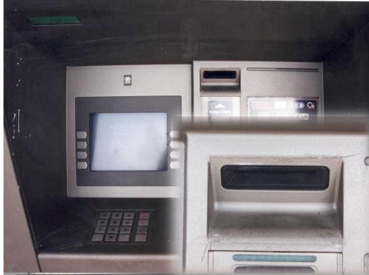
ATM skimmer (UK) Inset shows card skimmer attached in front of machine card slot.
