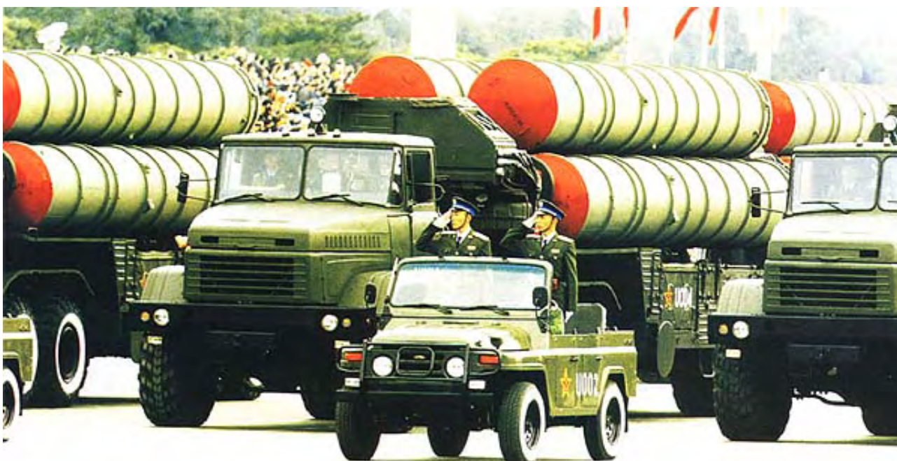
Figure 36: The PLA uses the SA-10 as a replacement for the obsolete S-75 system, reversed engineered by Chinese industry as the HQ-2, and available in semimobile variants and full mobile variants. US sources claim that a licenced SA-10 variant, the HQ-9, is being manufactured in China. The HQ-9 is the basis of the FT2000 anti-radiation missile, designed to destroy Airborne Early Warning and Control aircraft (PLA).
