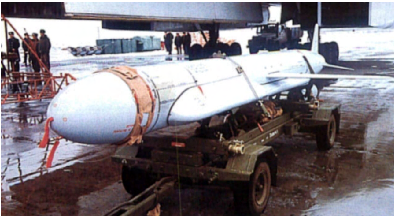
Figure 40: The Raduga Kh-55 Granat or 'Tomahawk-ski' (AS-15 Kent) cruise missile was developed as an equivalent to the US AGM-86 carried by the B-52H and the US RGM-109 Tomahawk carried by submarines, and arms the Tu-95MS and Tu-160 strategic bombers. Numerous reports claim the PLA illegally acquired Kh-55 rounds from the Ukraine five years ago, and legally purchased tooling for the non-nuclear Kh-65 variant of this missile. The lower image shows the improved Kh-55SM with conformal fuel tanks, providing a range of up to 1,600 nautical miles (RuMoD).
