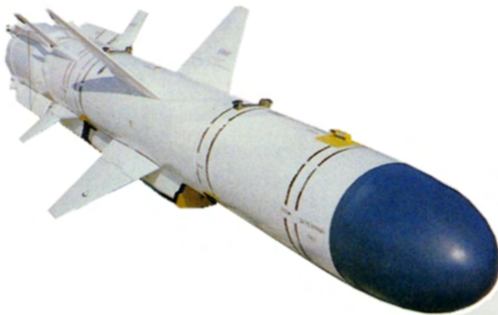
Figure 47: The Kh-59M/D series stand-off weapon is a direct equivalent to the AGM-142 missile now being integrated on the RAAF's F-111C, and carried by the US B-52H (Upper). Evolved from an anti-radar missile, it is now available with an optical seeker. The PLA-N is reported to have ordered an anti-ship variant equipped with a radar seeker, designated the Kh-59MK2 (-). Dubbed the 'Kharpunski' the Kh-35U Uran is the Russian equivalent to the US RGM-84/AGM-84 Harpoon carried by the F-111C and RAN warships (Lower). The missile is available in surface launched and air launched versions (Rosvooruzheniye).
