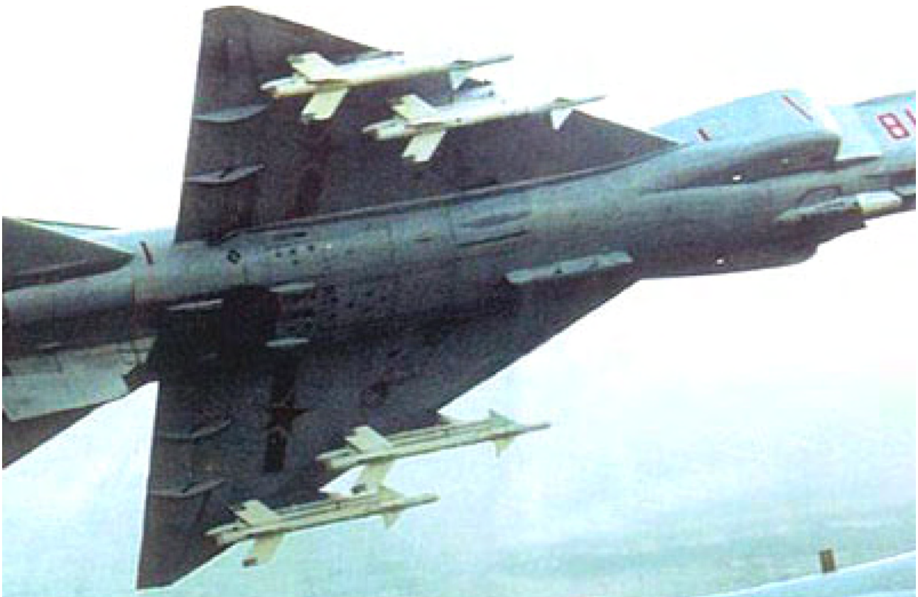
Figure 30: The J-8-II Finback B is an indigenous Chinese multirole fighter and is broadly equivalent to the Russian Su-15/21 series and RAF Tornado ADV/IDS. The lower image depicts a J-8-II armed with PL-8 missiles, reversed engineered from the Israeli Python 3 (PLA).
