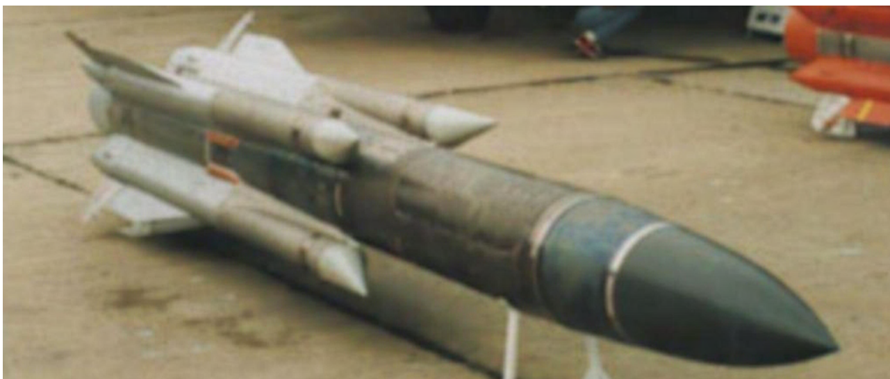
Figure 46: The supersonic ramjet Kh-31P was originally designed as an anti-radar missile to suppress NATO air defences. Since the end of the Cold War it has evolved an extended range variant, the Kh-31MP, and an anti-ship variant equipped with a radar seeker, the Kh-31A/MA. It has no equivalent in the Western inventory. The PLA is reported to have licenced this weapon (RuMoD).
