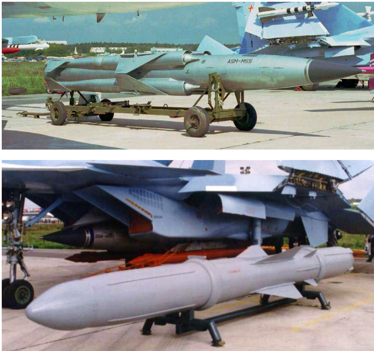
Figure 42: Raduga Kh-41/3M-80/3M-82 Moskit (Upper). This supersonic sea skimming anti-ship cruise missile has been exported to the PLA in its ship-launched variant. The missile is on offer as the air launched Kh-41 for the Su-30MK fighter. There is no Western equivalent to the Moskit (Rosvooruzheniye). OKB-52 3K-55/3M-55 Yakhont (Lower). This supersonic sea skimming anti-ship cruise missile has been licenced to India for domestic manufacture. It has been reported as the armament for latter 956E series destroyers to be supplied to the PLA-N. There is no Western equivalent to the Yakhont/Brahmos (Rosvooruzheniye/NIC).
