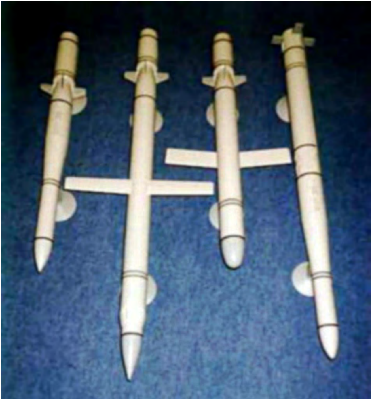
Figure 43: Novator 3M-54 Alfa/Club. This family of subsonic and supersonic sea skimming anti-ship cruise missiles has been exported to the PLA. The Club suite includes the subsonic 3M-54E1 anti-ship and 3M-14E land attack missiles which resemble a shortened Tomahawk, and the supersonic 3M-54E anti-ship missile. The Club is available in ship-launch, submarine-launch and air-launch variants, the submarine-launch variant is now in service. The land attack 3M-14E recently entered production. There is no direct Western equivalent to the 3M-54E (Rosvooruzheniye/NIC).
