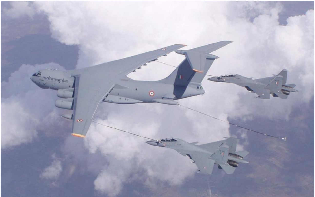
Figure 6: India is taking delivery of its first Il-78MKI tankers, a type being widely marketed across the region. This example is refuelling a pair of advanced Su-30MKI fighters. With aerial refuelling the Sukhoi fighters can significantly extend their prodigious combat radius, which without refuelling is around 60% greater than that of the RAAF's F/A-18As (Indian Air Force).
