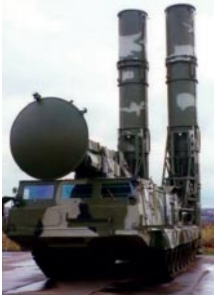
The S-300V/S-300VM/Antey-2500 is the world's only truly mobile Anti Ballistic Missile system, and later variants are claimed to be capable of intercepting 4.5km/sec re-entry speed targets. The large size of the Grill Pan phased array and TELAR command link and illuminator antennas is evident. The system provides the capability to engage very low RCS aircraft at ranges in excess of 100nm (185km). (Rosvooruzheniye)
