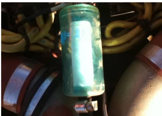
Figure 2: Empty fuel filter in engine bay.
