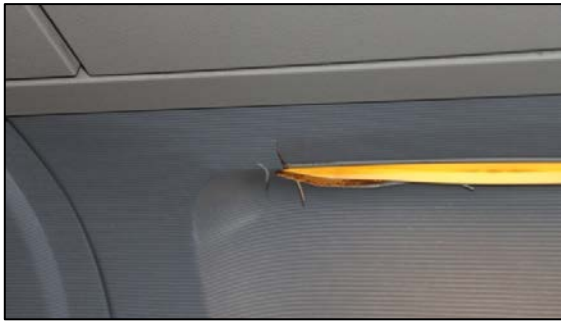
Figure 1: Damage to window reveal and overhead locker
