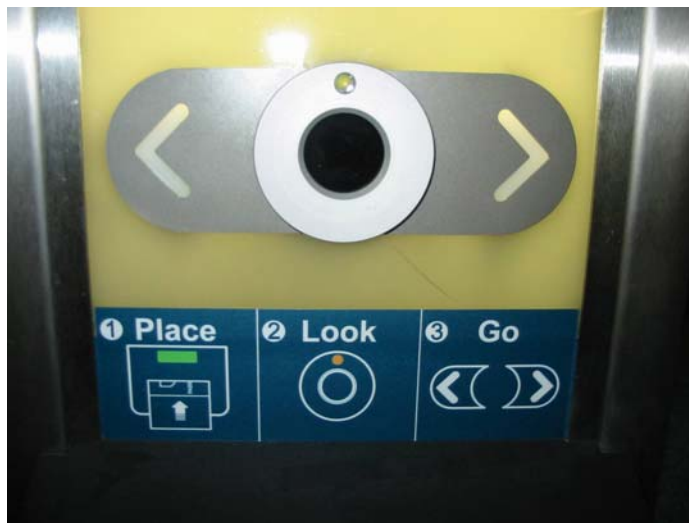
Photo 4: A blue arrow is located to the side of the camera, which becomes illuminated when the user is required to proceed to the Customs Officer for manual processing.
