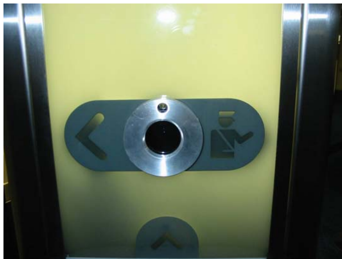
Photo 3: Each of the cameras is fitted with three signal lights. An orange light located centrally and to the top of the camera indicates that the cameras and data matching process are in operation. A green arrow is located to side of the camera, which becomes illuminated upon a successful transaction.
