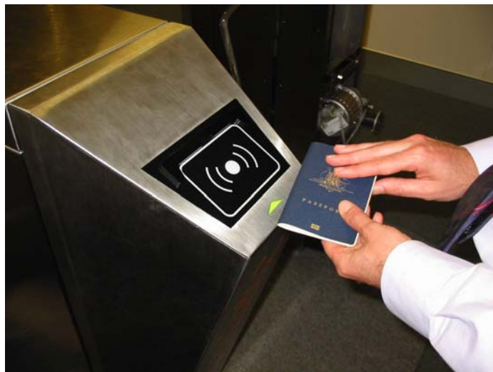
Photo 9: The placement of the passport to the passport reader. Note the green arrow to the base of the reader and the illuminated symbol to reflect passport placement.
