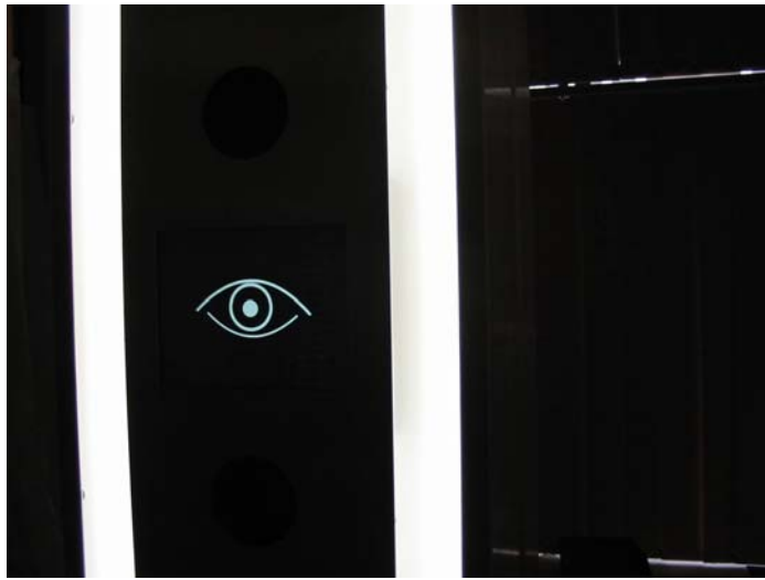
Photo 12: The LCD screen displays the symbol of an eye to indicate to the user to look at the cameras ahead
