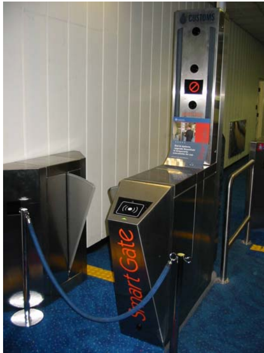
Photo 6: The cameras are located at three positions (approximately 1400, 1650 and 1900 mm above the floor)
