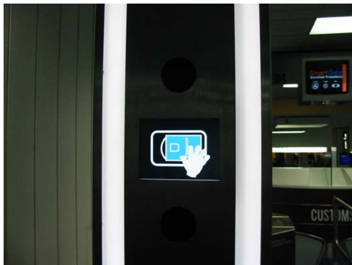
Photo 7: The LCD screen is positioned between the cameras positioned at 1400 and 1650 mm above the floor. This flashing two-stage instruction indicates the instruction to place the passport to the reader.
