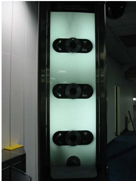
Photo 2: The cameras are located at three positions (approximately 1450, 1650 and 1850 mm above the floor)
