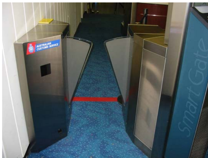
Photo 5: Upon receiving a green illuminated arrow indicator the user proceeds to the automatic gates for passage through the Customs Control point.
