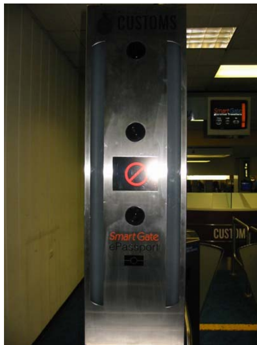
Photo 10: The LCD screen displays a red crossed circle symbol to indicate an unsuccessful passport read or non-operability of the kiosk
