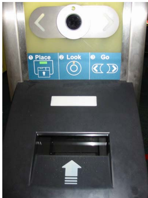
Photo 1: The placement of the passport to the passport reader is represented with an upward arrow symbol. The three-stage process is illustrated above the passport reader.
