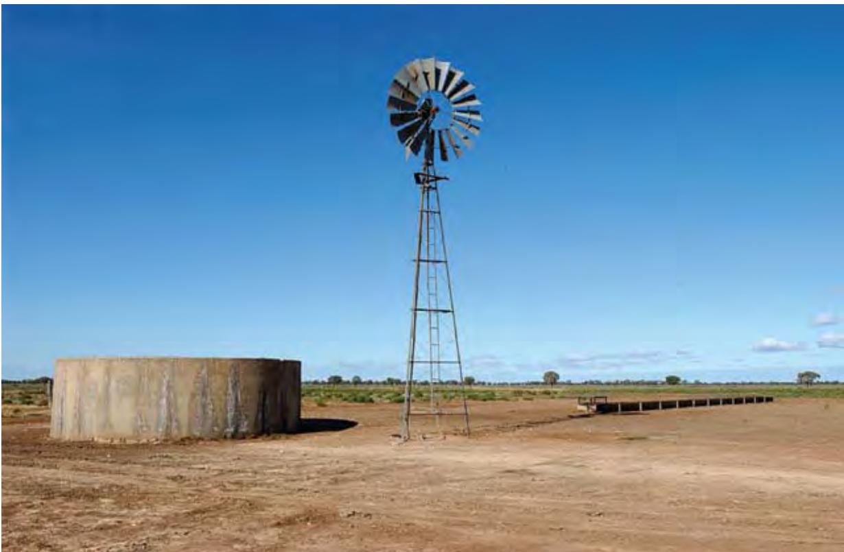
Windmill pumping groundwater for stock in Australia
