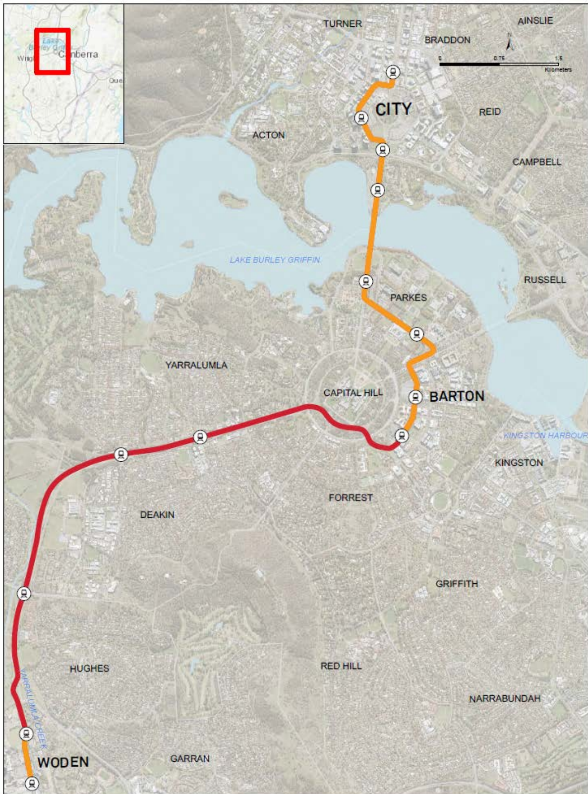
Figure 4.2 Overhead line power and wire-free running locations
