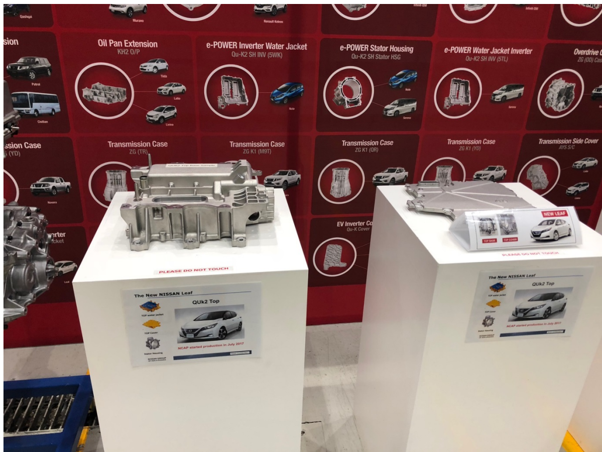
Photo 4: Examples of completed die-cast components
