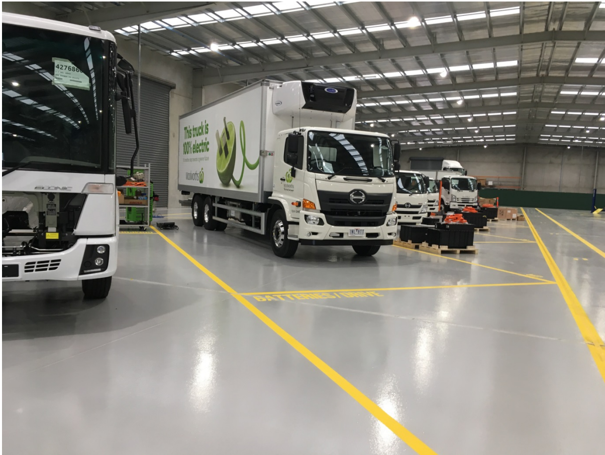
Photo 6: A number of gliders being fitted with EV powertrains and batteries in the SEA Electric workshop
