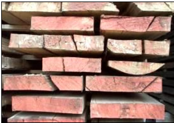
Board distortion, Stress and drying induced end split in sawn plantation-grown E. regnans – plantation E. globulus behaves similarly
