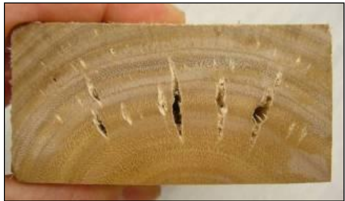
Internal check in dry 11 year old plantation E. nitens – not a problem for structural wood but will cause void or pick problems with fine finishing
