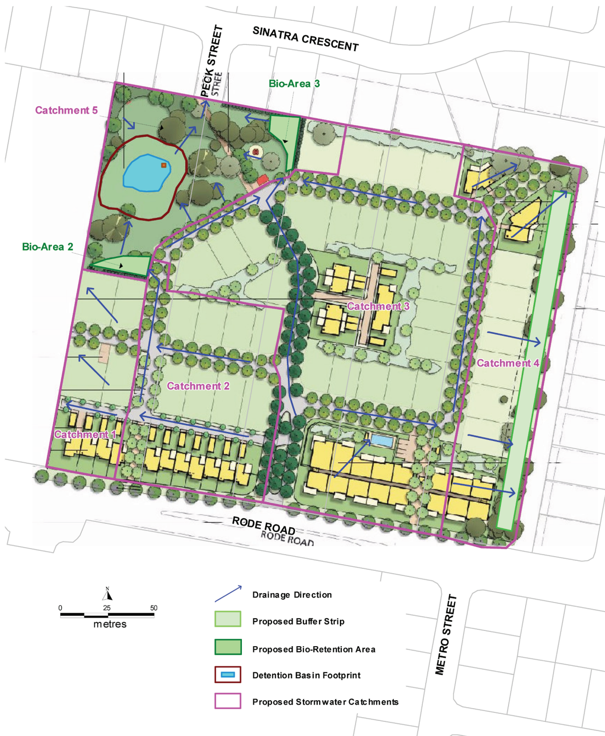
Figure 2.1 Proposed Site Layout with Stormwater Drainage
