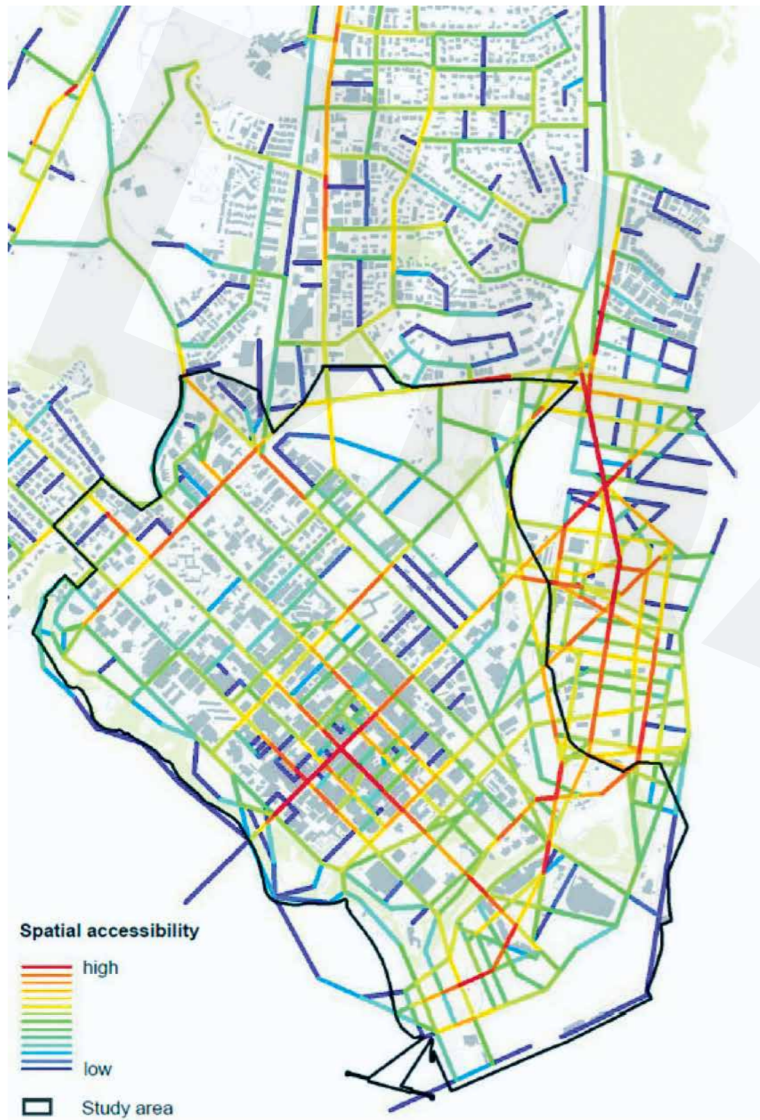
Figure 84 – Model forecasting walkability based on spatial accessibility and walking evidence (Space Syntax Limited)
