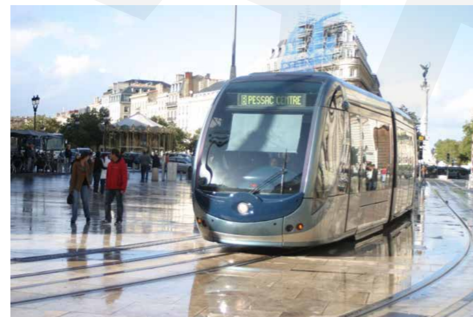
Fig. 58 - Light rail without overhead cables. Bordeaux, France, servicing a population of 200,000 people
