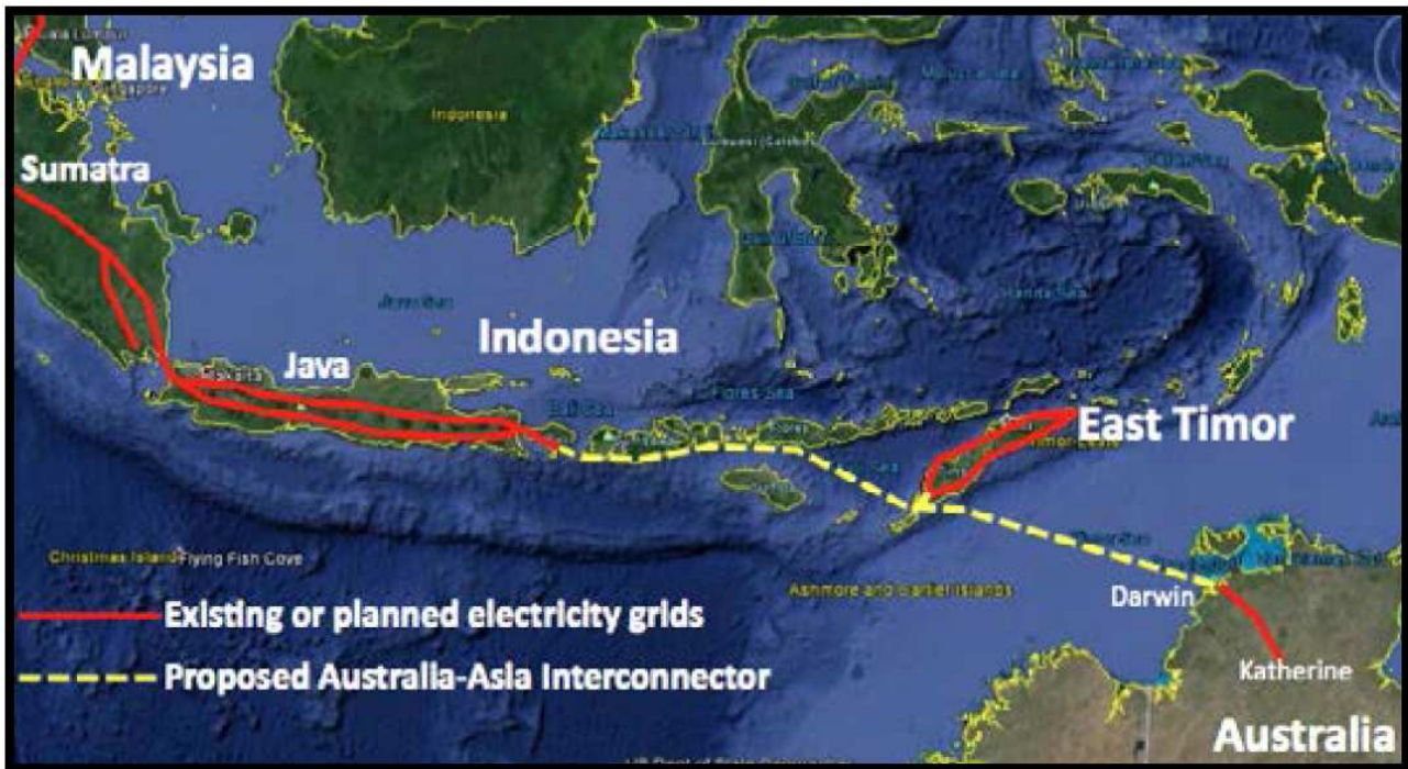
Figure 4. Proposed Australia-Asia Interconnector joining the electricity grids of the Top End, Timor and western Indonesia. A High Voltage Direct Current subsea cable would enable electricity generated from renewable energy to be exported from Australia to Asia.
