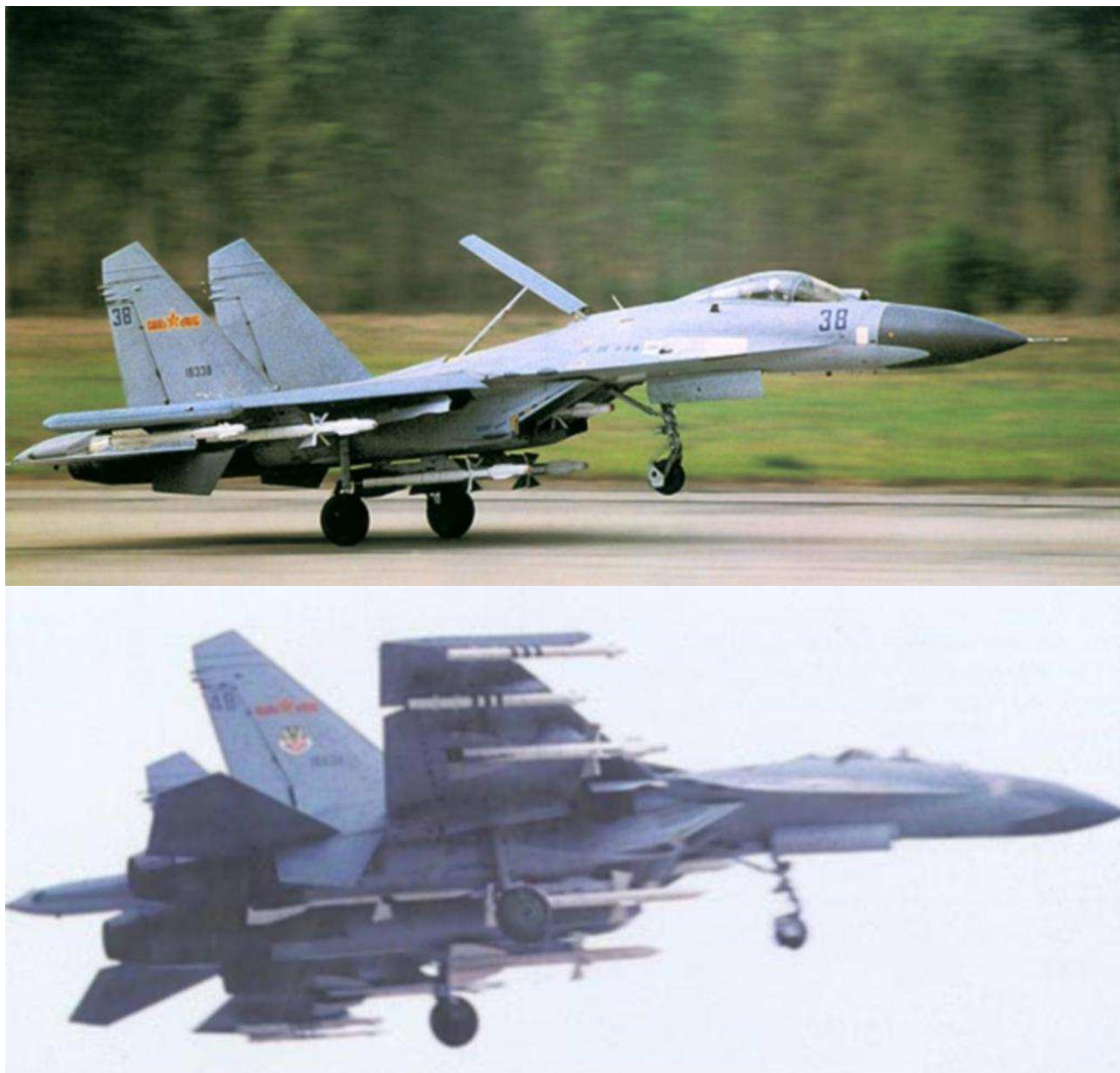
Figure 7: The KNAAPO/Shenyang J-11 is an imported or licence built Russian Su-27SK long range multirole fighter, broadly equivalent to the US F-15C Eagle. Current planning sees around 300 in service by 2015 (PLA).
