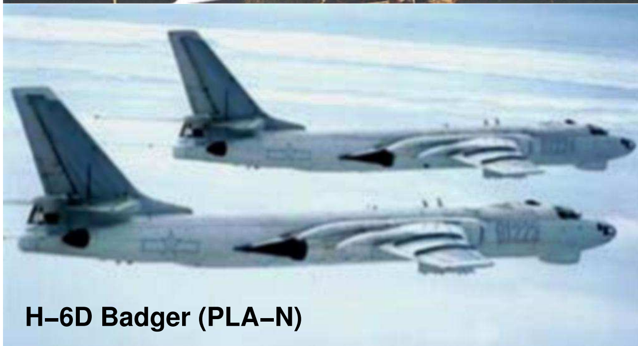
Figure 9: The Xian H-6 is a reverse engineered Russian Tu-16 Badger, broadly equivalent to the 1960s RAF V-bombers. Around 150 are in service, mostly built between 1972 and 1992 (PLA).
