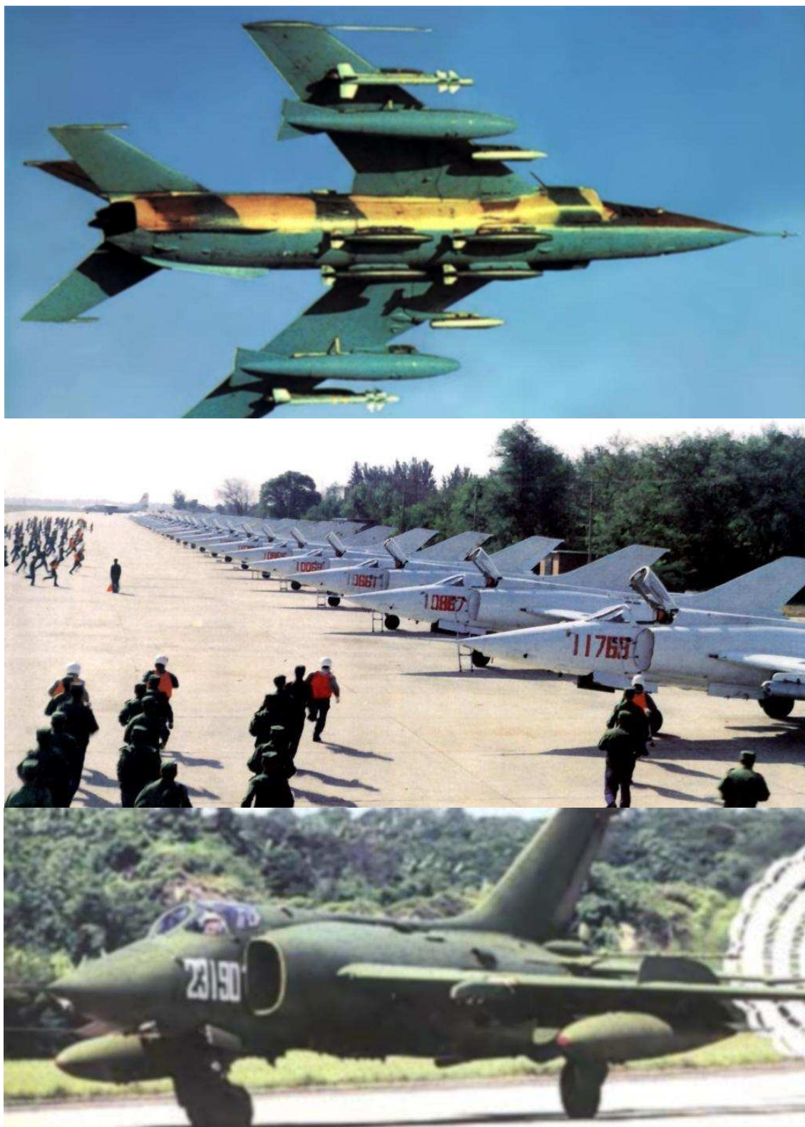
Figure 1: Q-5 Variants. The Q-5 is an indigenous evolution of the Russian MiG-19 Farmer and is broadly equivalent to the A-4 Skyhawk. Around 600 are in service (PLA).
