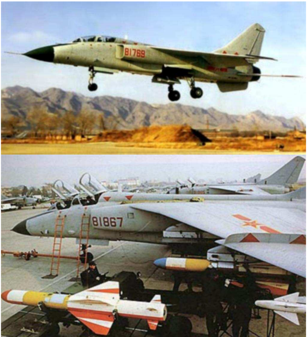
Figure 4: The Xian JH-7 is an indigenous Chinese strike fighter and is broadly equivalent to the RAF Tornado IDS. Around 20 serve with the PLA naval air arm (PLA).
