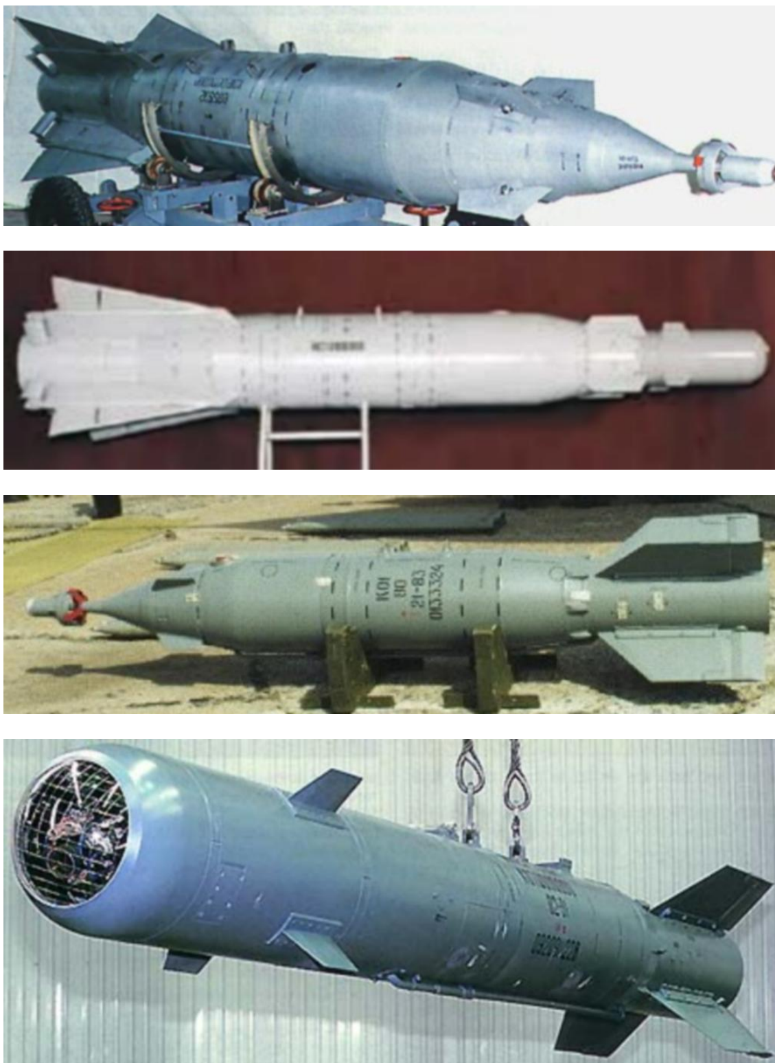
Figure 16: Russia is actively marketing smart bombs for the Sukhoi fleets supplied to Asian nations. These images depict the laser and television guided KAB-1500 (1500 kg) series and KAB-500 (500 kg) series guided bombs, available in bunker busting and standard explosive variants. These weapons are broadly equivalent to the US Raytheon GBU-10, GBU-24 carried by RAAF F-111s, and the Boeing GBU-15 which was carried by the F-111 during the 1980s (Rosvooruzheniye).
