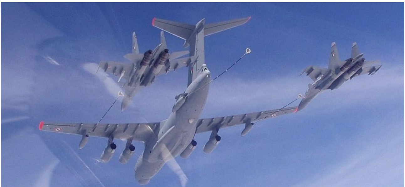
Figure 17: India recently took delivery of its first Ilyushin Il-78MKI aerial tankers from the CIS. This aircraft is the most capable non-Western tanker in service. This example is refuelling two Su-30MKI fighters (IAF).
