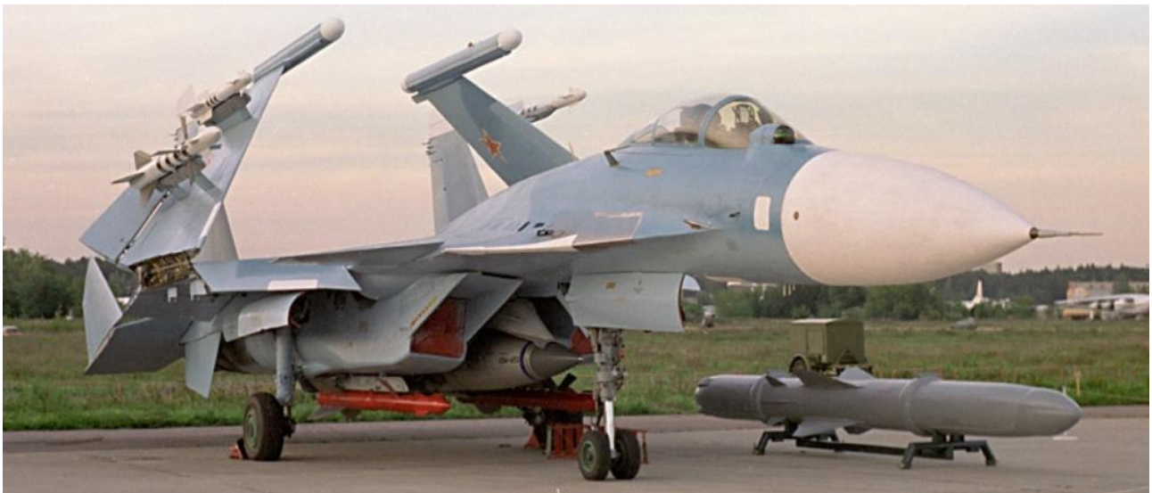
Figure 15: The NIIP BARS (N-011M) phased array radar (upper) fitted to India's Su-30MKI is the largest phased array carried by any third generation fighter, and is highly competitive against the newer technology APG-63(V)2 phased array radar fitted to some US F-15C fighters (NIIP). India has licensed the Russian Yakhont supersonic cruise missile (lower right), to be produced under the name 'Brahmos'. This missile will be available in anti-ship and land attack models (NIIP, S. Lavrov).
