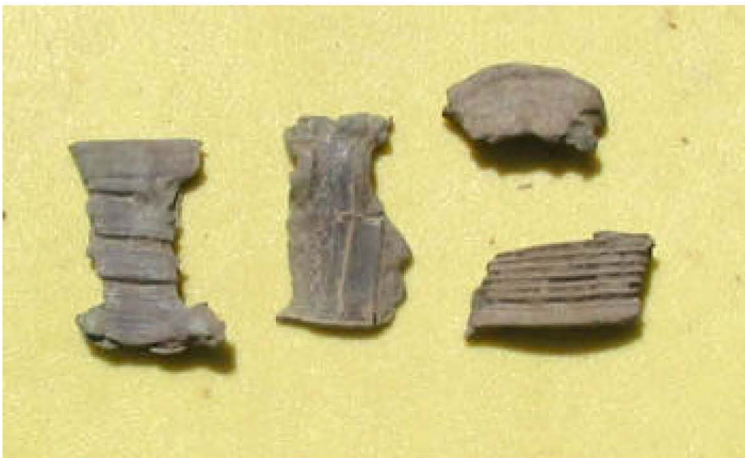
Photograph 10. Finds – Portions of projectile driving bands and components from functioned military fu zes.
