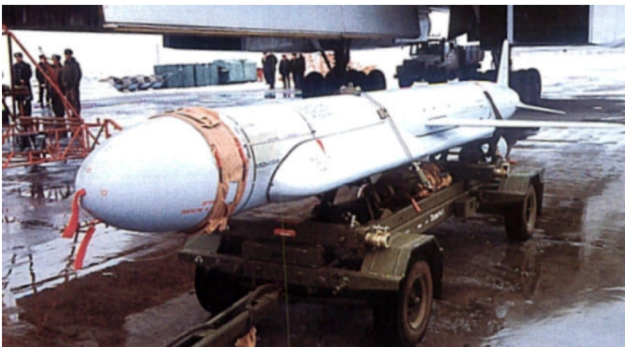
Figure 12: The Raduga Kh-55/55SM Granat or 'Tomahawk-ski' (AS-15 Kent) cruise missile was developed as an equivalent to the US AGM-86 carried by the B-52H and the US RGM-109 Tomahawk carried by submarines, and arms the Tu-95MS and Tu-160 strategic bombers. Numerous reports claim the PLA illegally acquired Kh-55 rounds from the Ukraine, and legally purchased tooling for the non-nuclear Kh-65 variant of this missile (RuMoD).
