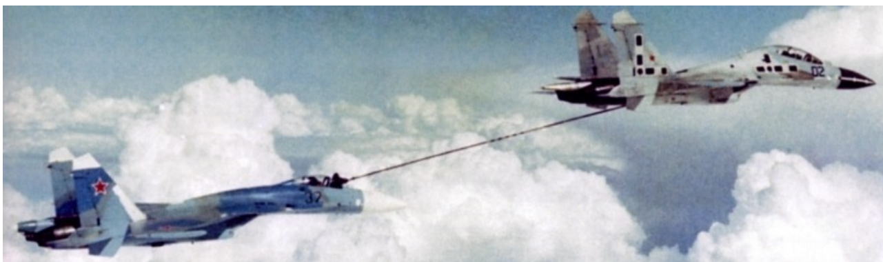
Figure 19: The Il-78MK Midas tanker uses a variant of the UPAZ-1A Sakhalin aerial refuelling pod, which has also been cleared for buddy refuelling on some variants of the Su-27 fighter (RuMOD).
