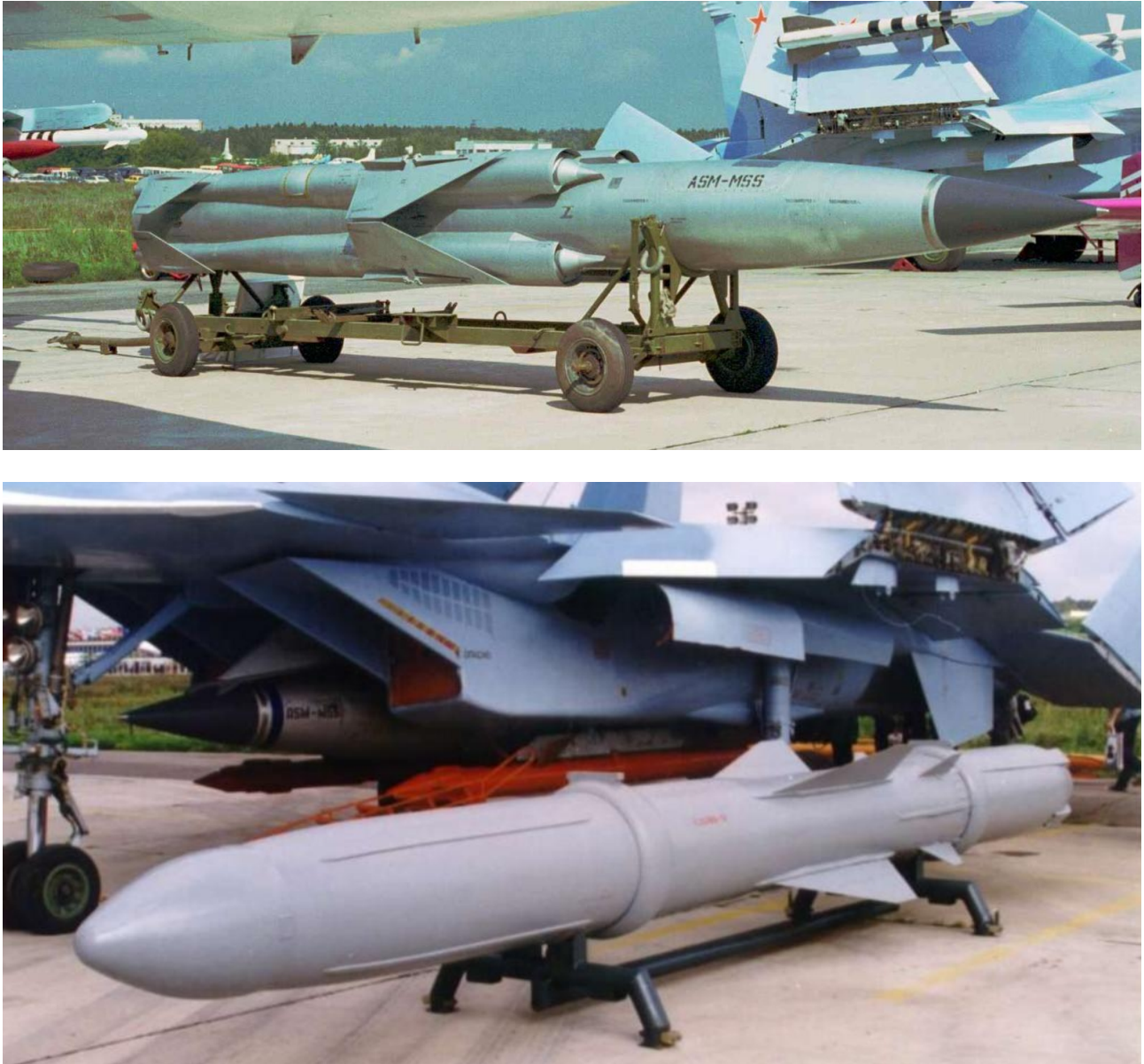
Figure 15: Raduga Kh-41/3M-80/3M-82 Moskit (Upper). This supersonic sea skimming anti-ship cruise missile has been exported to the PLA in its ship-launched variant. The missile is on offer as the air launched Kh-41 for the Su-30MK fighter. There is no Western equivalent to the Moskit (Rosvooruzheniye). OKB-52 3K-55/3M-55 Yakhont (Lower). This supersonic sea skimming anti-ship cruise missile has been licenced to India for domestic manufacture. It has been reported as the armament for latter 956E series destroyers to be supplied to the PLA-N. There is no Western equivalent to the Yakhont/Brahmos (Rosvooruzheniye/NIC).
