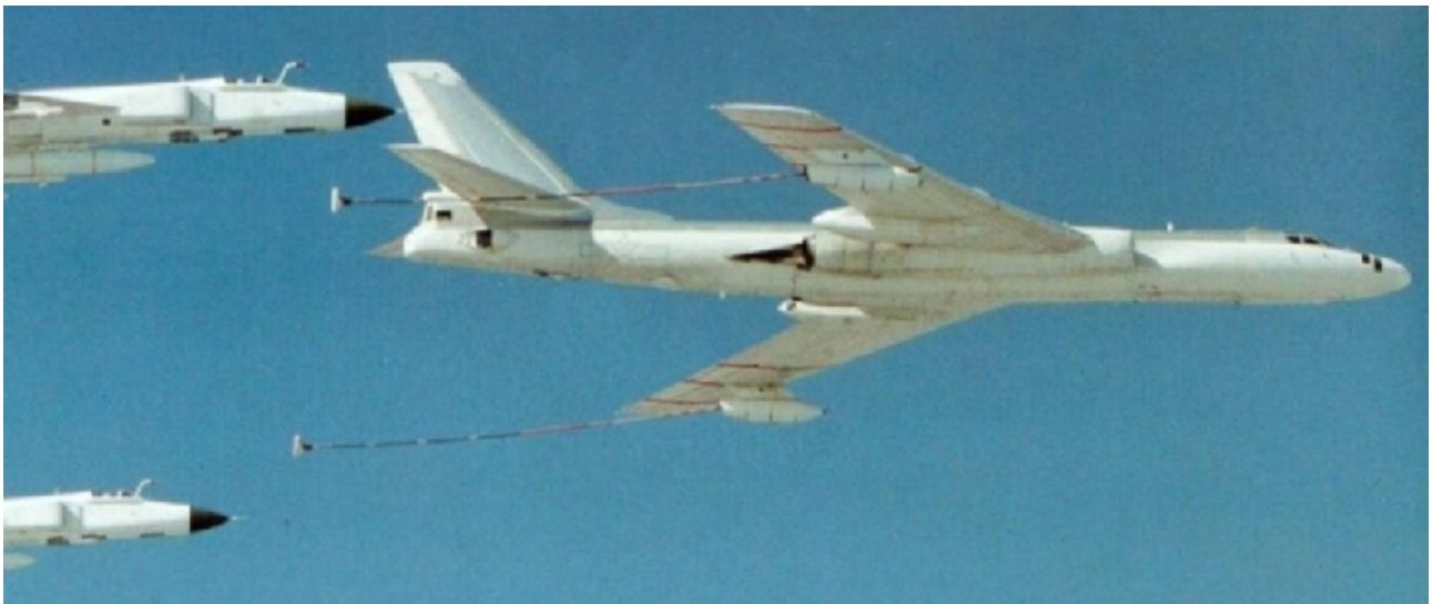
Figure 20: The Xian H-6 is the basis of China's indigenous aerial refuelling tanker program. Development was reported to be initially a collaboration with Flight Refuelling Limited in the UK during the 1980s. With the questionable usefulness of the Badger as a strike aircraft, it is likely many more will be converted to tankers, especially given the low age of much of the Badger fleet. As a tanker the Badger compares closely to the now retired RAF Victor K.2 (PLA).
