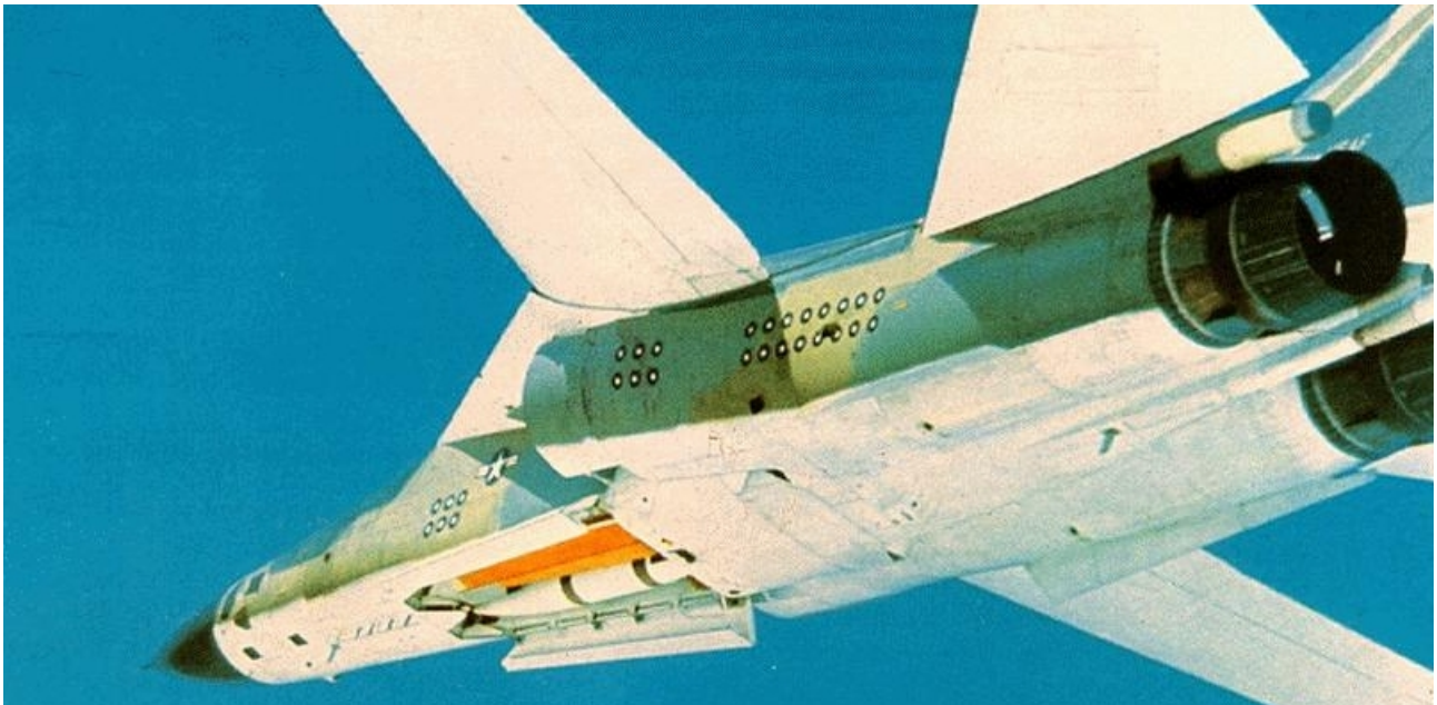
Figure 10: The USAF FB-111A employed the internal weapon bay for the B43, B57 and B61 nuclear weapons, while around 50% of the FB-111A fleet was configured to launch the 2,230 lb AGM-69A SRAM missile from the bay (US Air Force).
