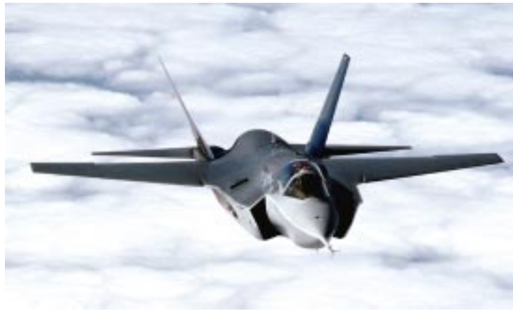
Both the F/A-22A and JSF use similar planform alignment and stealth shaping rules, reflecting a common design heritage. In the critical forward sector, the much more refined design of the F/A-22A is evident especially in the edge aligned inlet configuration and cleaner chining. The F/A-22A scatters into a smaller number of lobes over a much wider frequency band, reflecting its all aspect 'wideband' stealth requirement. (USAF & LM)
