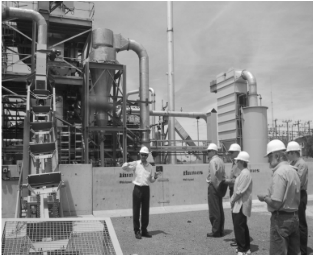
Photograph 6.1 Use of mallee eucalypts as a preventative treatment for salinity, and for concurrent production of eucalyptus oil, activated carbon and electricity in a bioenergy (demonstration) plant constructed by Western Power Corporation, at Narrogin in Western Australia
