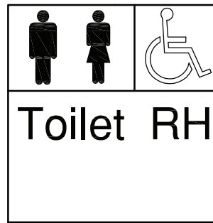
(c) Example of a sign identifying accessible facility indicating right hand transfer (RH) (Left hand transfer-LH)
