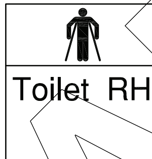
(d) Sign identifying a compartment for people with ambulant disabilities with the appropriate symbol
