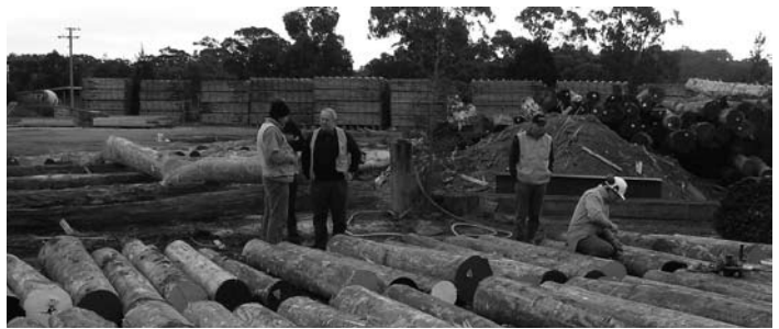
Logs are colour coded so that sawn boards can be identified during processing trials.
