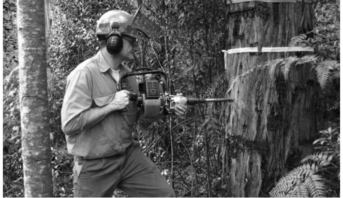
Wood core samples collected in the field can be assessed for cellulose content and pulp yield using portable, hand held NIR spectroscopy.
