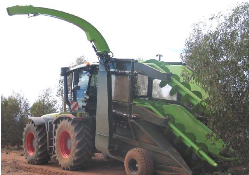
Prototype continuous mallee harvester undergoing field trials
