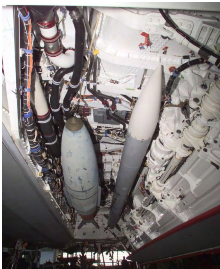
Figure 4: The F-22A Raptor (upper), can carry a pair of GBU-32 JDAM satellite/inertially guided precision bombs internally. The weapon is wholly autonomous once released and can attack targets through cloud, unlike laser guided bombs which are limited to clear weather conditions. Recently developed enhancements include a radio datalink which permits the JDAM to be used against moving targets such as ground vehicles or shipping. The JDAM proved itself convincingly in Serbia, Afghanistan and Iraq (US Air Force).
