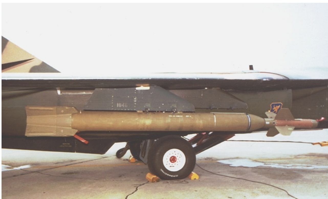
Figure 24: One of the valuable consequences of the F-111's size is its capability to carry large special purpose munitions like this GBU-28/B 'Deep Throat' bunker busting bomb. Smaller aircraft are unable to operate with weapons of this size. Despite the vital importance of this capability, the RAAF has no plans to introduce it and will lose that option if the F-111 is retired (US Air Force).
