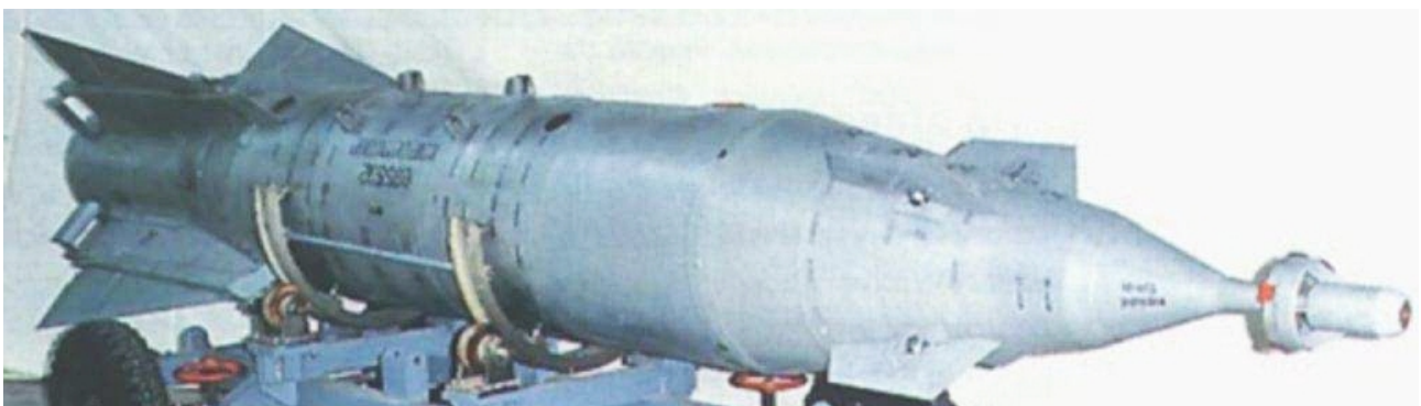
Figure 9: Precision Guided Bombs or 'smart bombs' have proliferated globally since the end of the Cold War, with US, Israeli, French and Russian products now widely available. Within the region, the Russian KAB-500 and KAB-1500 series are now widely deployed. These bombs combine the best aerodynamic features of the US GBU-8, GBU-10 and GBU-15 weapons, with laser, television, thermal imaging or satellite guidance. Warheads include blast, bunker busting, fuel air explosive and most recently, thermobaric designs (Legion.ru).
