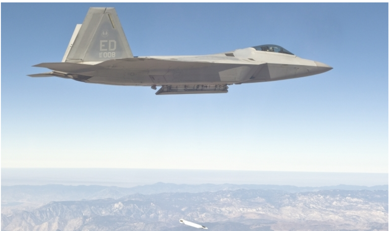
Figure 16: The stealthy supercruising F-22A Raptor will become the backbone of the US Air Force. The F-22A will escort non-stealthy and stealthy strike aircraft in high threat environments, defeating opposing fighter and surface based missile defences, and strike at high value heavily defended surface targets. The F-22A is regarded to be an “unstoppable” bomber, armed internally with a pair of GBU-32/B JDAM satellite inertial guided bombs (above), or up to eight GBU-39/B SDB glidebombs (US Air Force).
