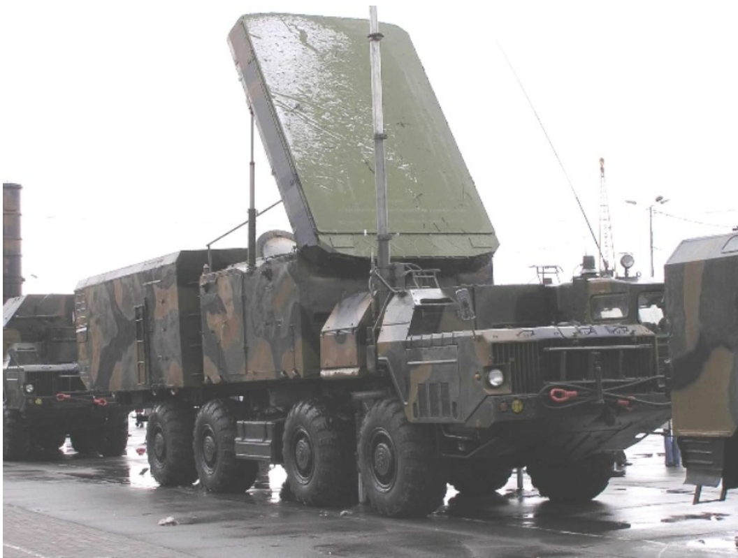
Figure 12: The high mobility NIIP 64N6E2 Big Bird is an acquisition radar with similar capabilities to the naval SPY-1 Aegis system (upper). The high mobility 30N6E2 engagement radar is the Russian equivalent to the Patriot MPQ-65 (lower), (Almaz-Antey).
