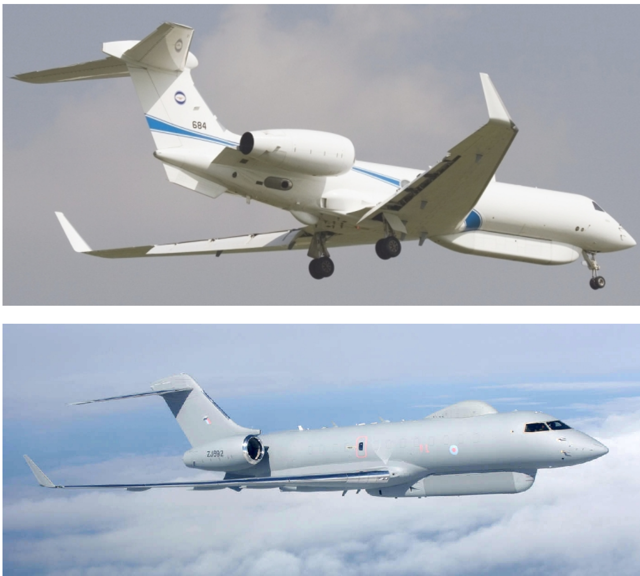
Figure 30: Potent electronic reconnaissance suites are now available in the market. This Israeli G550 system is an example (upper). The RAF's new Sentinel R.1 is a compact affordable X-band ground surveillance radar system (IAI, RAF).
