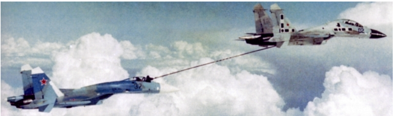
Figure 7: An option available on several Flanker variants is a buddy refuelling system, allowing the Flanker to act as an aerial refuelling tanker aircraft. Regional nations which cannot afford dedicated tanker aircraft have the option of emulating the US Navy practice of using fighters as buddy refuellers (KnAAPO).
