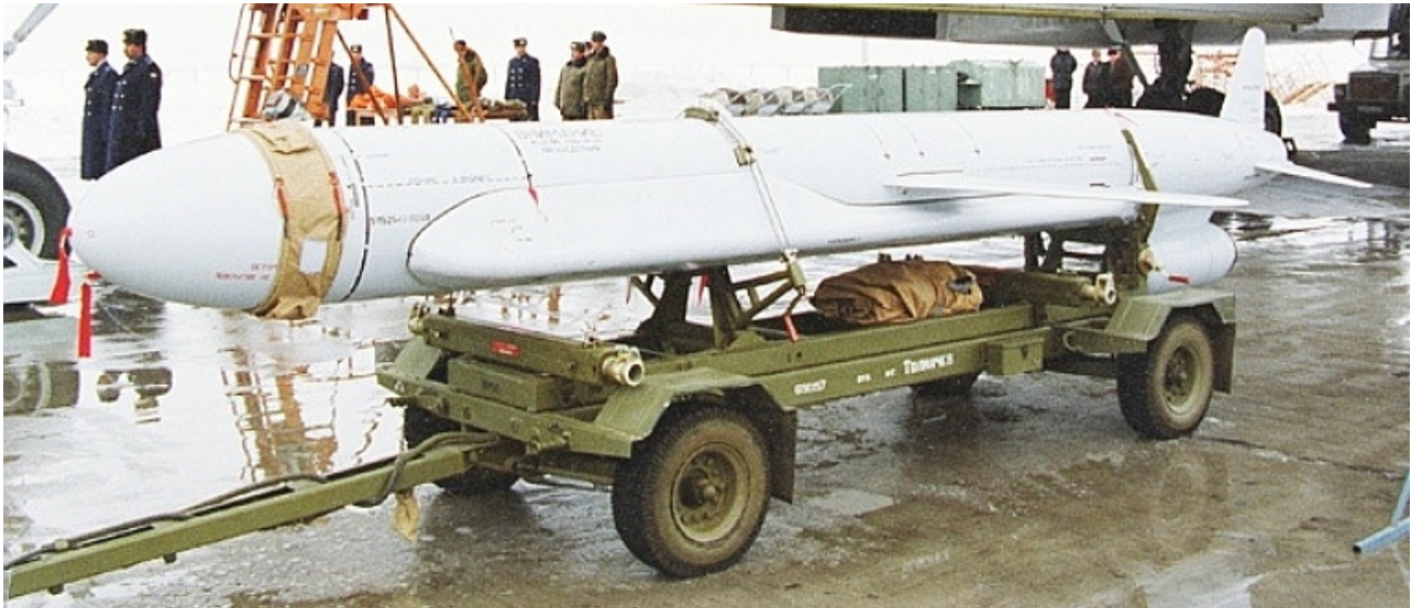
Figure 10: Raduga Kh-55SM Granat / AS-15 Kent cruise missile with conformal fuel tanks (RuMoD).
