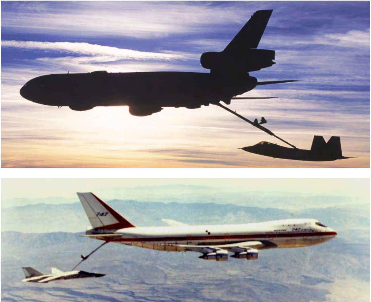
Figure 31: Aerial refuelling tankers are the critical enabler for fighter aircraft. In practical terms the number of fighters usable in most combat situations is determined by the number of aerial tankers available, rather than fighters on the flightline. In situations where range and endurance matter, such as Australia's north, heavy tankers are more suitable than medium sized tankers, such as the A330-200 ordered for the RAAF. Upper - US Air Force KC-10A heavy tanker, lower - prototype ACTA heavy tanker based on the 747 (US Air Force).
