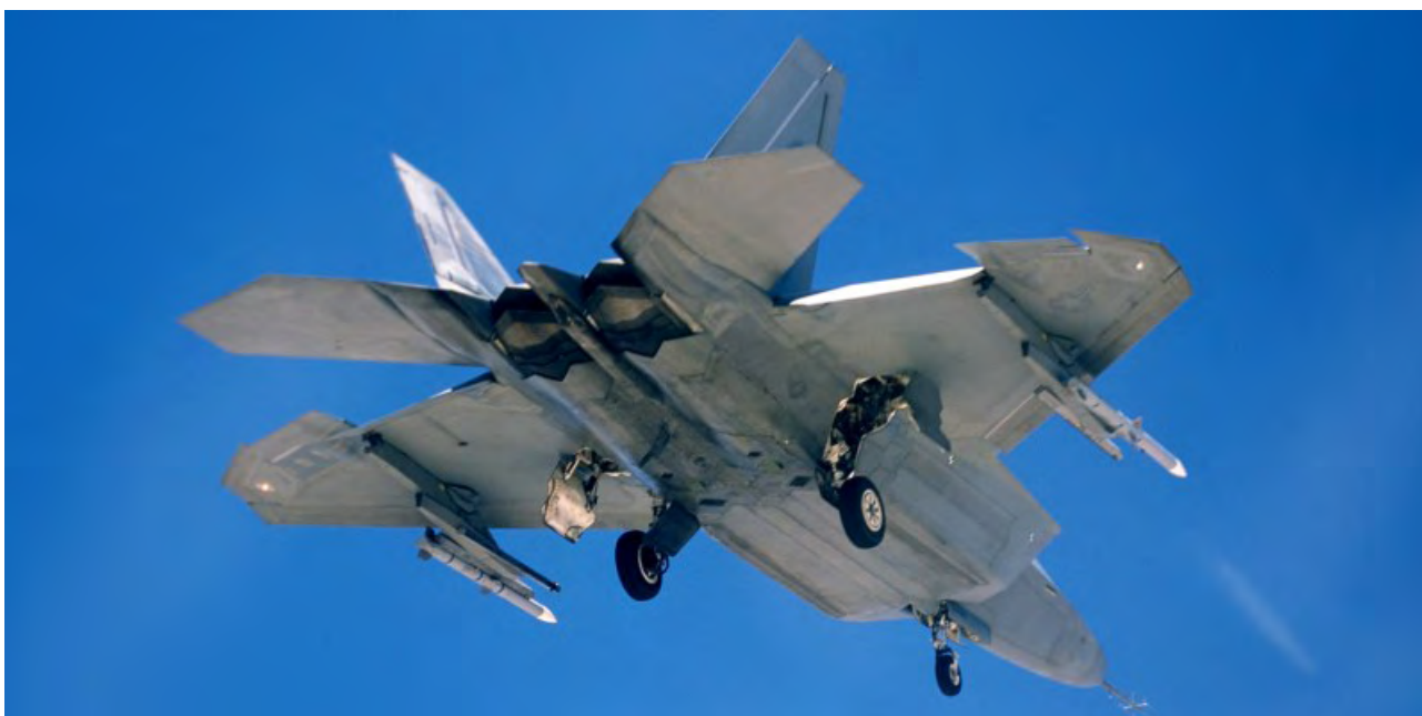
Figure 45: An early production F-22A Raptor releasing a GBU-32 JDAM satellite aided guided bomb (upper). The F-22A is a true multirole fighter, intended to excel in the air superiority role, but also to attack the most heavily defended surface targets with precision guided munitions. With unchallenged survivability it will also be used for electronic and imaging radar reconnaissance. The F-22A is designed to carry internal weapons where stealth is required, but can also carry significant external payloads where stealth is not required (lower) (US Air Force).
