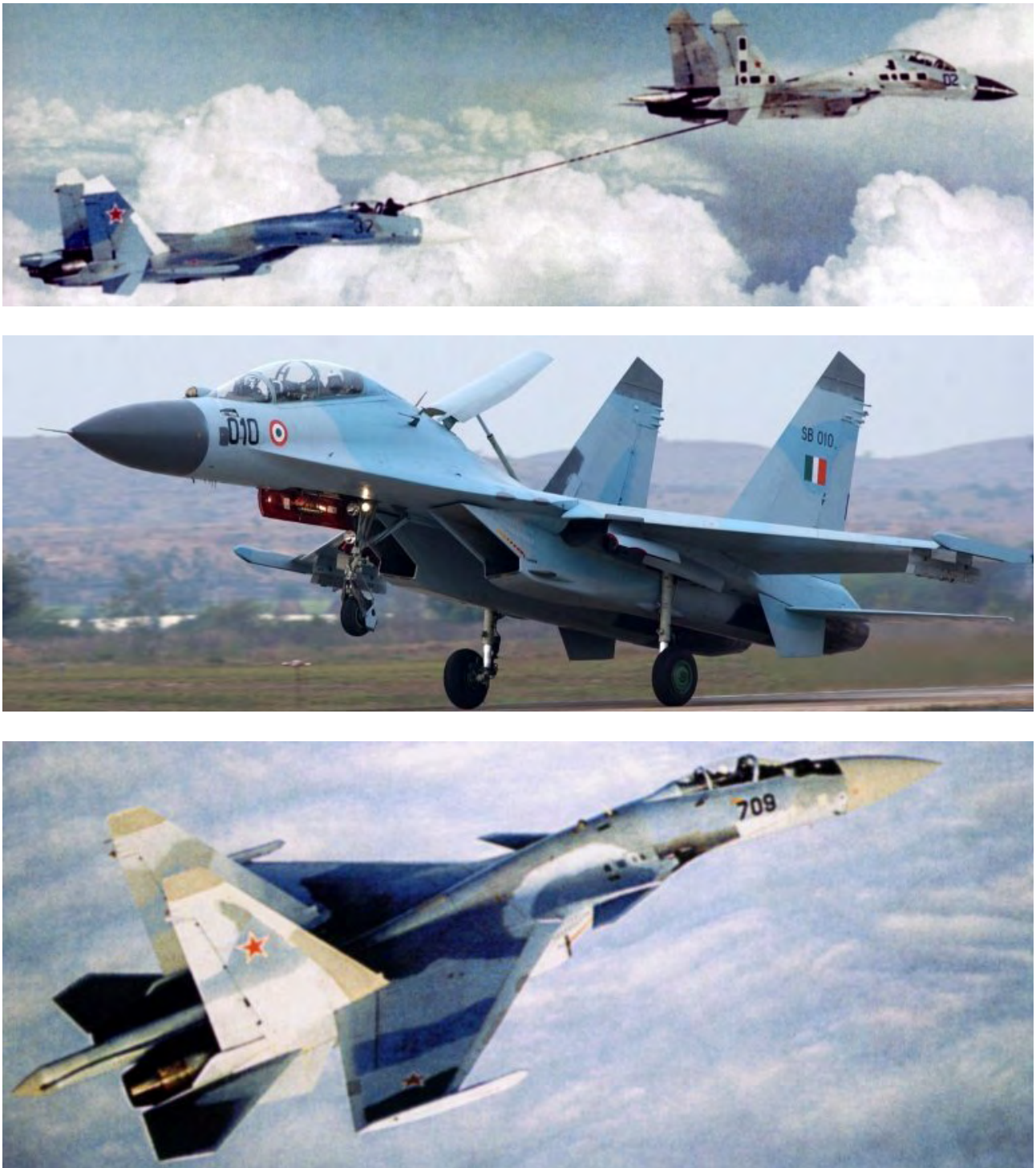
Figure 11: Advanced Flanker variants such as the Su-27SMK Flanker B, Su-33 Flanker D, Su-30MKI/MKK/MKM Flanker G/H and Su-35 Flanker E have key capabilities in common with modern US and EU fighters. These include aerial refuelling probes, buddy refuelling pods, advanced multi-mode radar strike modes, electro-optical targeting systems, digital network modems, glass cockpits and the capability to carry a wide range of smart munitions (Sukhoi, US Air Force).
