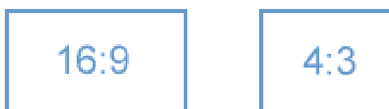
Figure 1.1 Aspect ratios of widescreen television and traditional analogue television.
