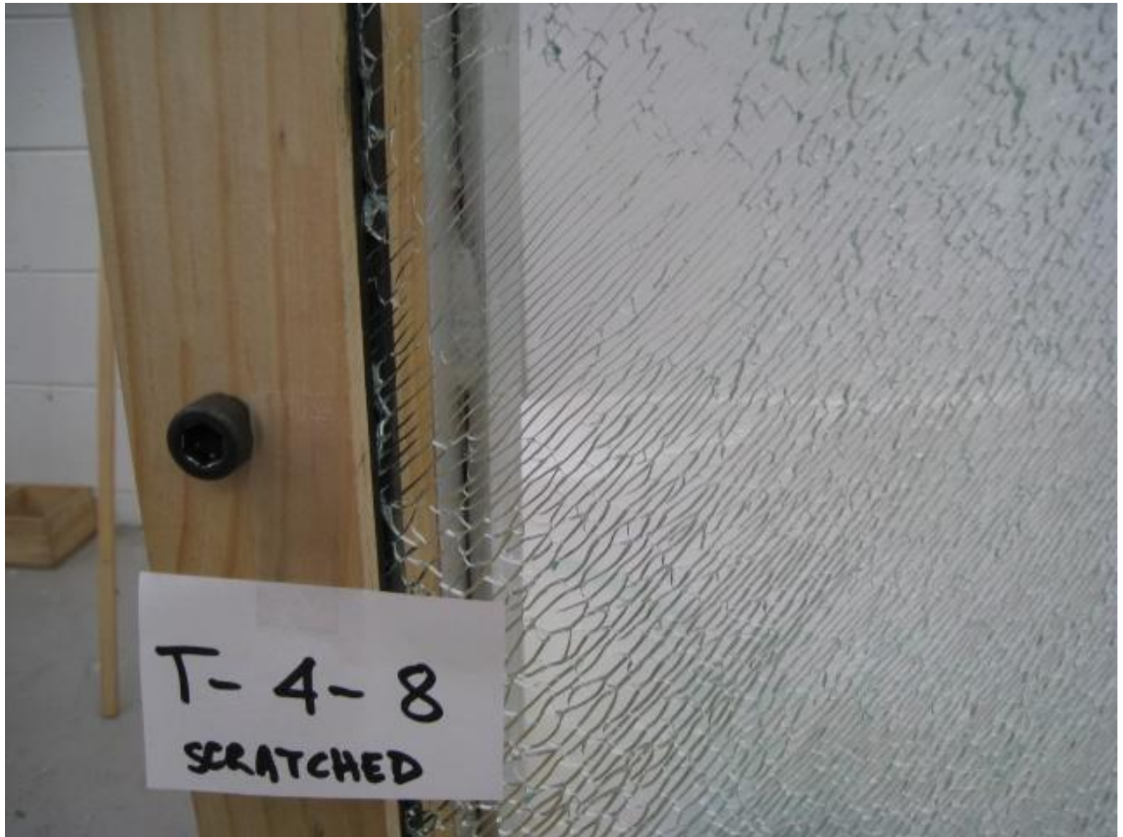
4 mm Sample No.1_4-8; SC 100 MPa: LSB - Glass in frame
