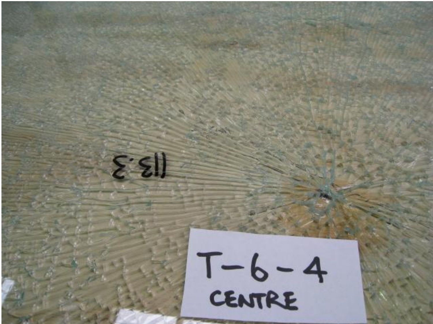
6 mm Sample No. 1_6-4; SC 113: Centre Fragmentation - Longest Particle 100 mm
