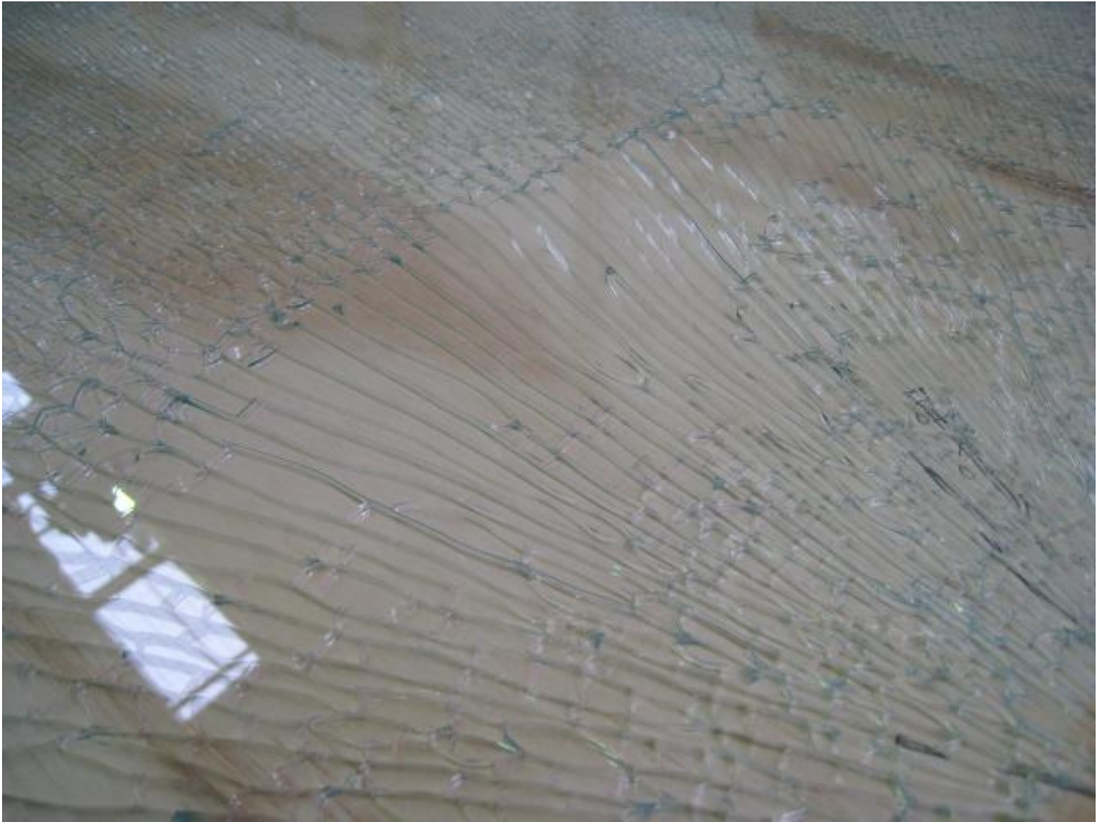
4 mm Sample No.1_4-6; SC 113: Centre Fragmentation, Longest Particle 170 mm
