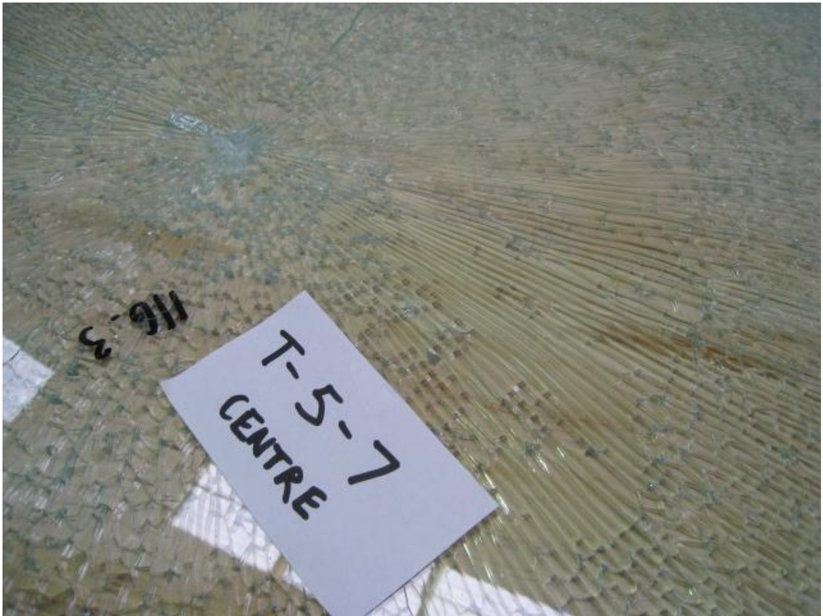
5 mm Sample No.1_5-7; SC 116; Centre Fragmentation - Longest Particle 151 mm
