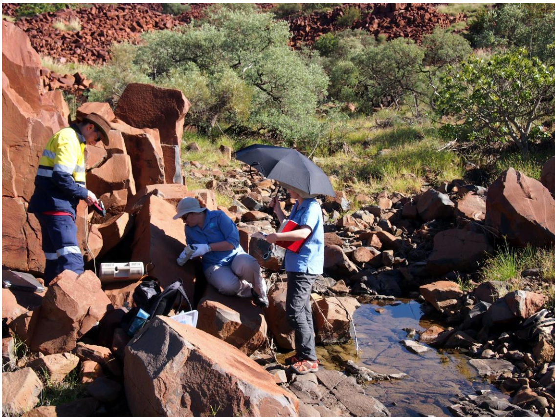
Figure 16: ASD FieldSpecPro and Konica Minolta CM-700dspectrophotometer operating on petroglyphs in the Burrup Peninsula (2013)
