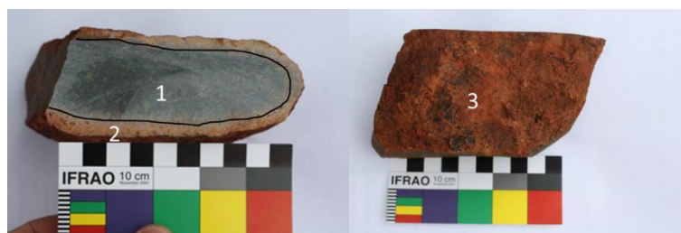
Figure 3. Weathered granophyre with Munsell colour including (1) fresh rock (7.5B 5/2), (2) leached zone (7.5YR 4/2) and (3) surface coating (2.5YR 4/4).
