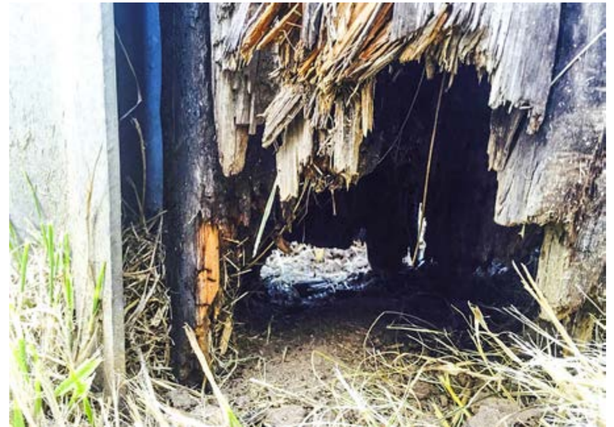
ⓐ Pole in service - completely rotten on ground.
