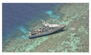
electronic chart display and information system (ECDIS) identified the reef as a danger to the planned route. However, the vessel's officers did not identify the danger, either visually or using the ECDIS. The investigation highlighted that the safe and effective use of ECDIS as the primary means of navigation depends on the mariner being thoroughly familiar with the operation, functionality, capabilities and limitations of the specific equipment in use on board their vessel.
