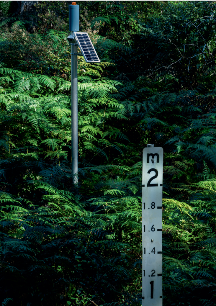
DipStik flood-monitoring system installed at Wedderburn causeway near Campbelltown in NSW (IAG, 2017)
