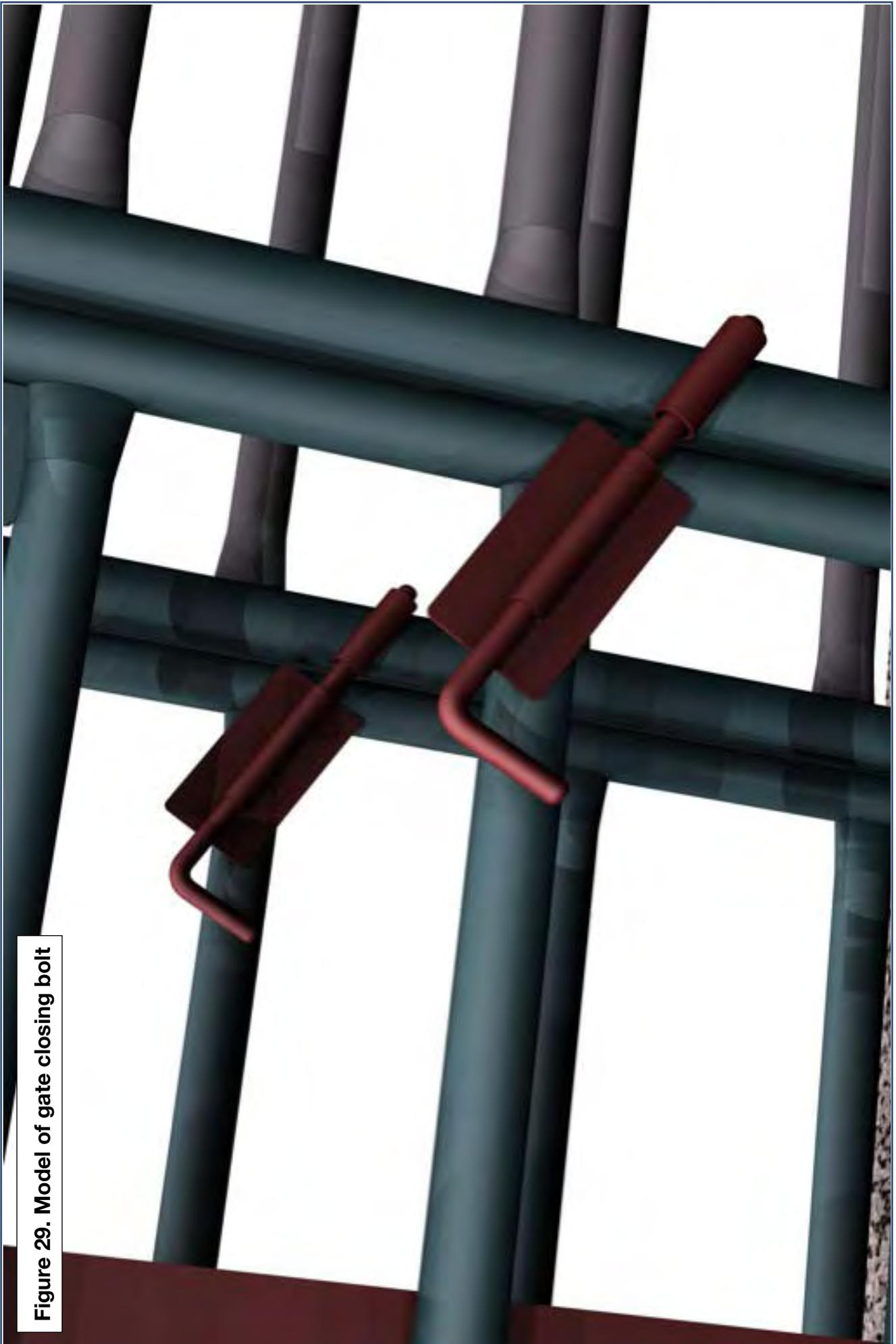
Figure 29. Model of gate closing bolt
