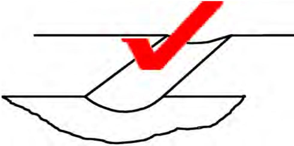
Spoon drains (spoon shaped) have no corners, therefore are an efficient means of moving solids and water away from yards for treatment.
