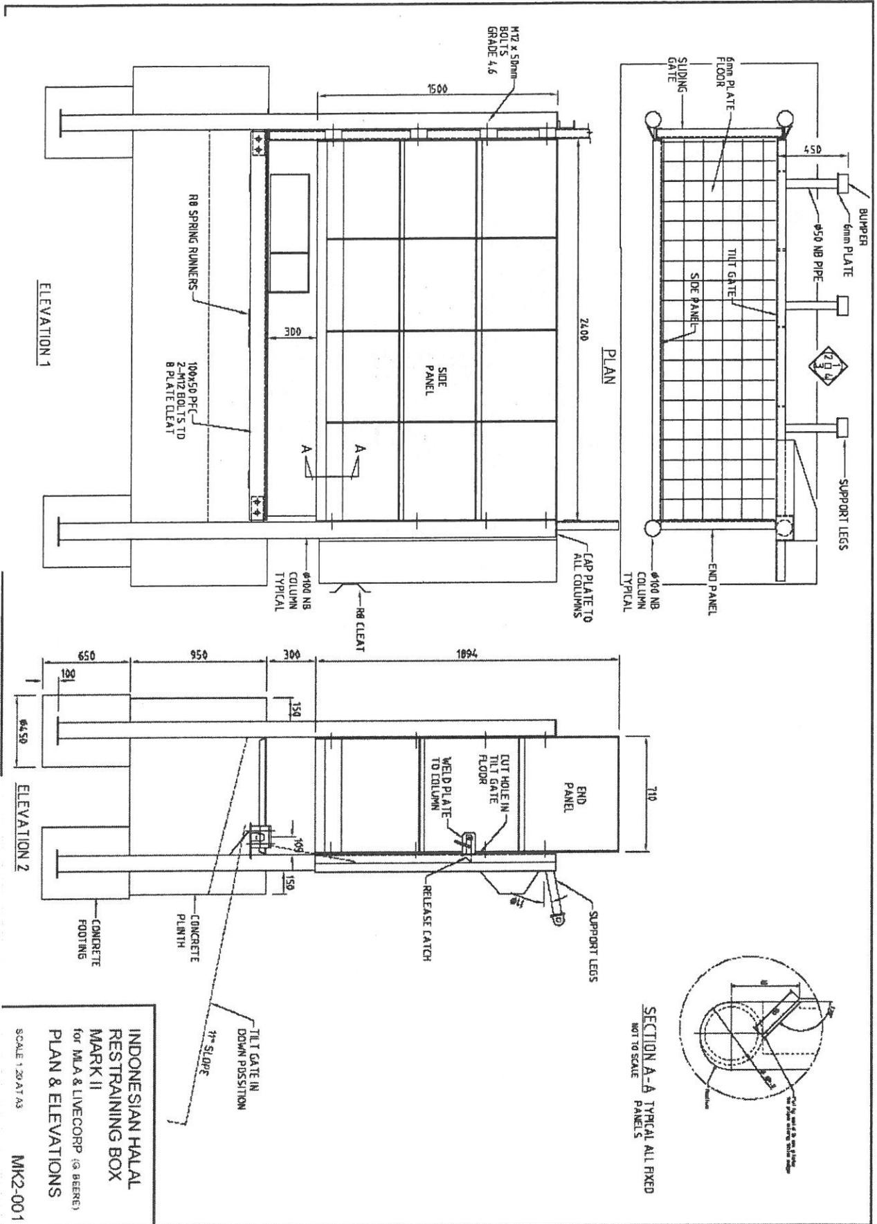
Figure 7.1 Mark 2 box plan & elevations
