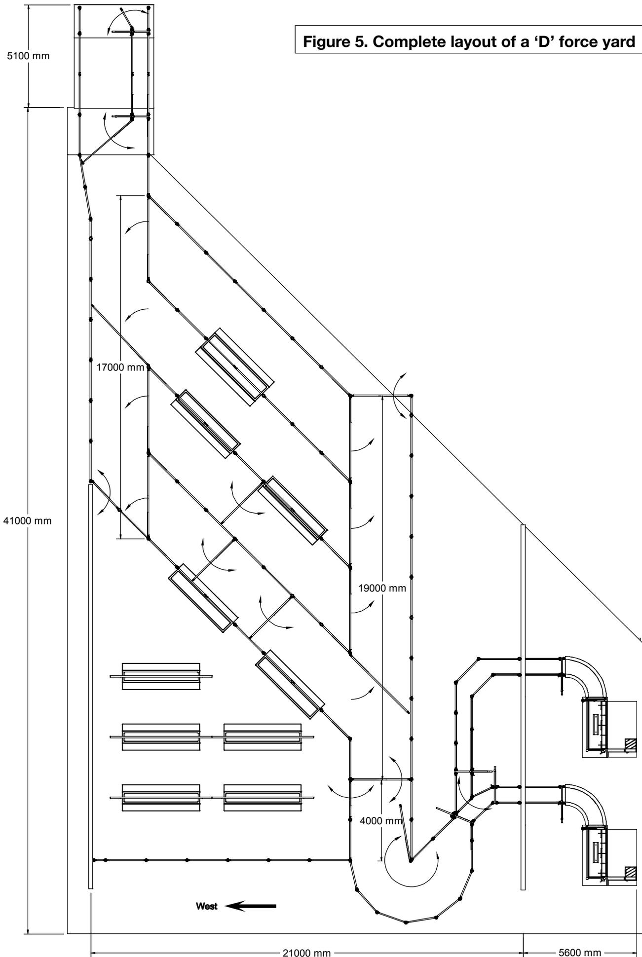
Figure 6. Model of a 'D' force pen
