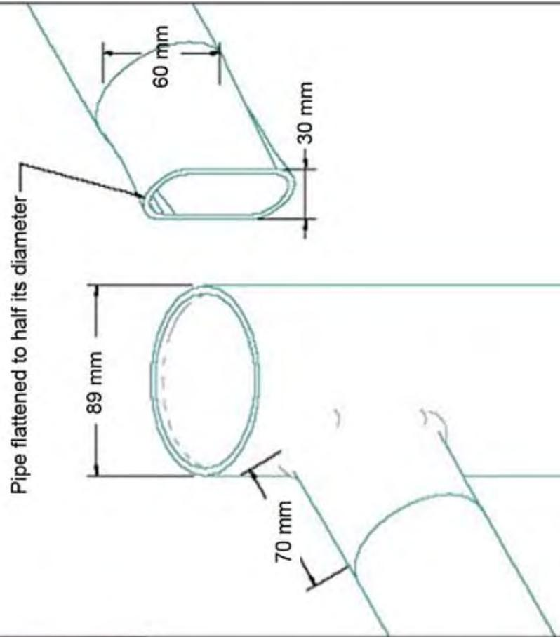
**Figure 31. Gate pivot details showing PVC pipe on posts**
