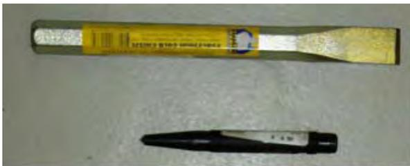
Tempered coal chisel
