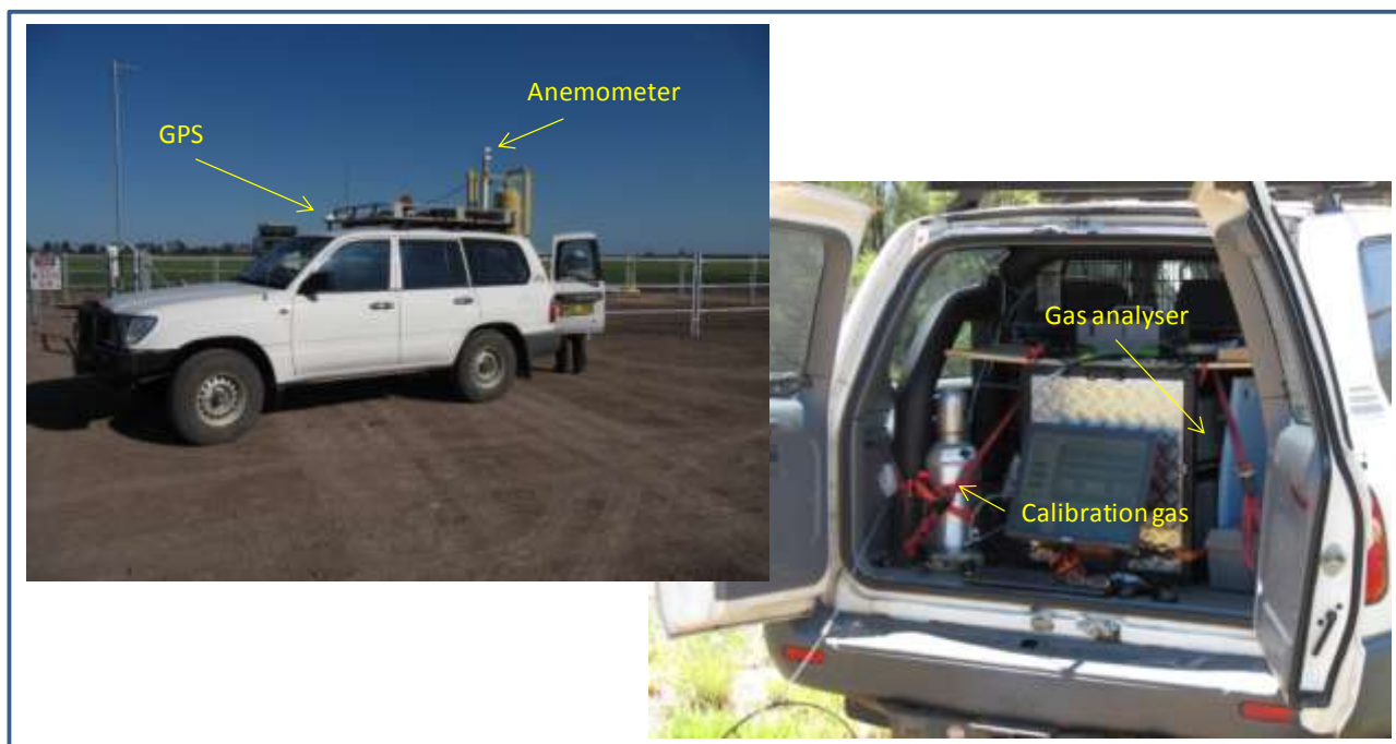
Figure 3.1. Photographs of the field vehicle where the GPS antenna and sonic anemometer are visible on the top of the vehicle (left hand photograph). The methane analyser and a calibration gas cylinder are shown in the rear of the vehicle (right hand photograph).
