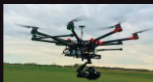
Figure caption: Sample of group 1 UAS capable of heavier payload modification. Higher-end group 1 UAS are modifiable for a range of payloads, including surveillance and explosive material.
