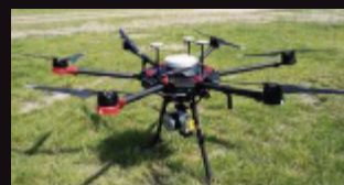
Figure caption: Sample of group 1 UAS capable of heavier payload modification. Higher-end group 1 UAS are modifiable for a range of payloads, including surveillance and explosive material.
