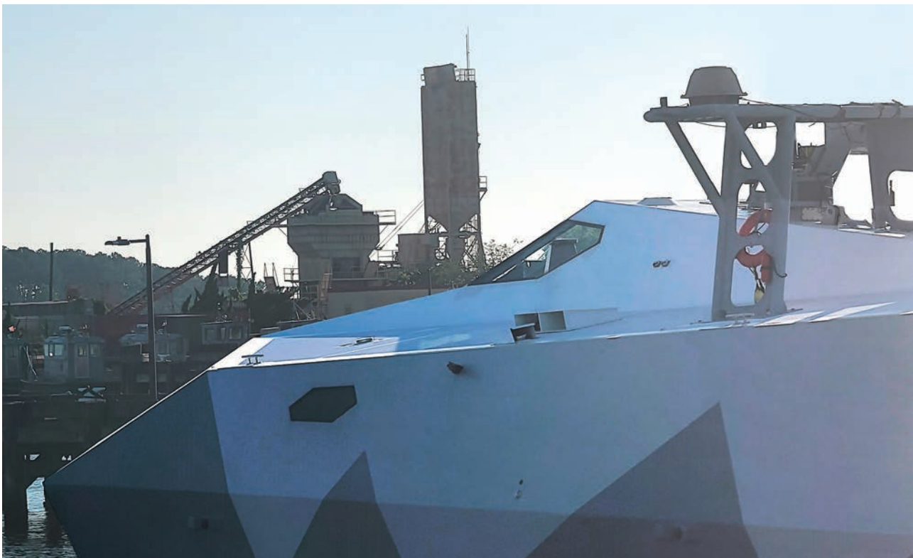
Photo caption DroneShield DroneSentry-X ship mounted direction-finding UAS sensor (using RF technology).
