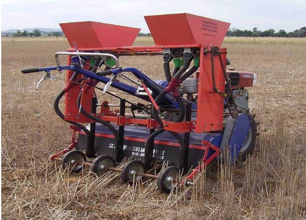
The ACIAR modified rotary tillage unit ready for testing in NSW, Australia. Photo: ACIAR
