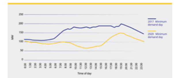
COMPARISON OF DEMAND PROFILE ON MINIMUM DEMAND DAY IN 2017 AND 2020 IN DARWIN-KATHERINE [MW]
