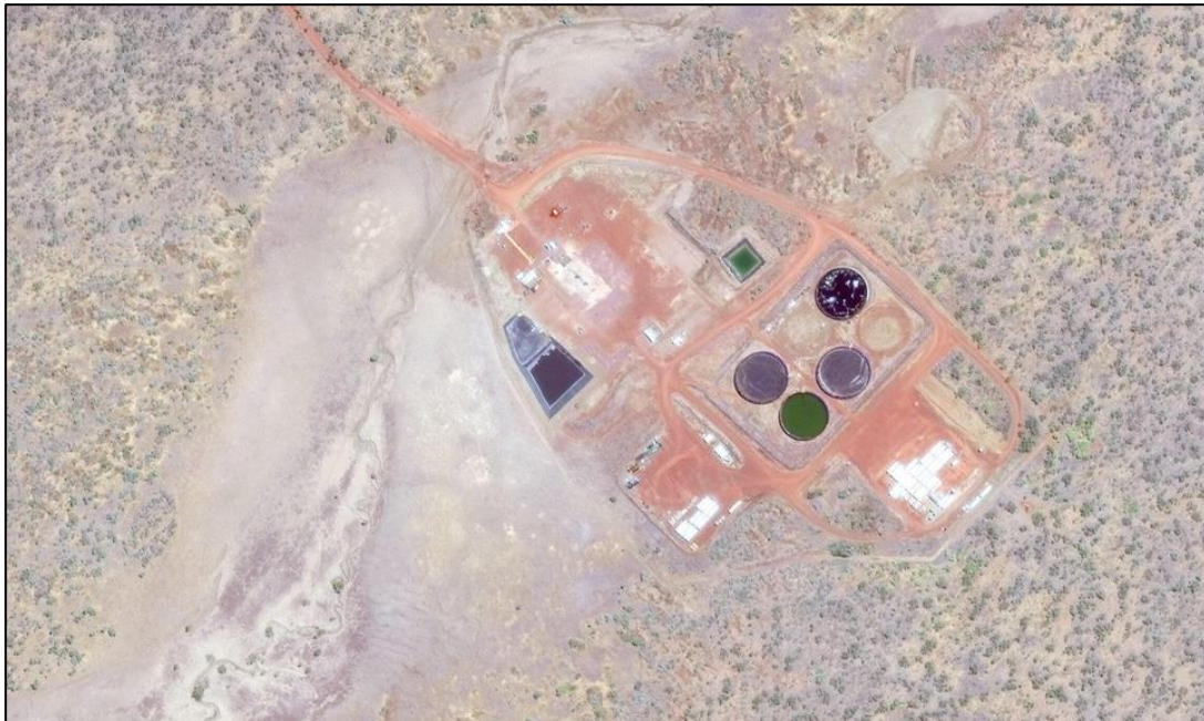
Aerial view of a single Beetaloo frack pad showing open evaporative ponds. SecureWatch2022 Maxar Technologies
