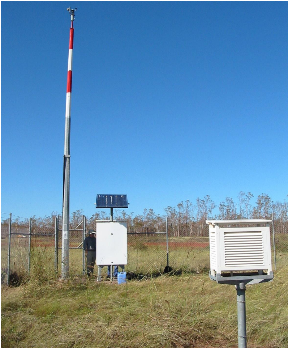
Figure 2.2.8 BoM’s weather station at Maningrida aerodrome. The cup anemometer is atop the 10 m high mast on left and an ‘Almos’ type AWS is in the white box beneath the solar panels. (Photograph is copyright Australian Bureau of Meteorology and is used with permission.)
