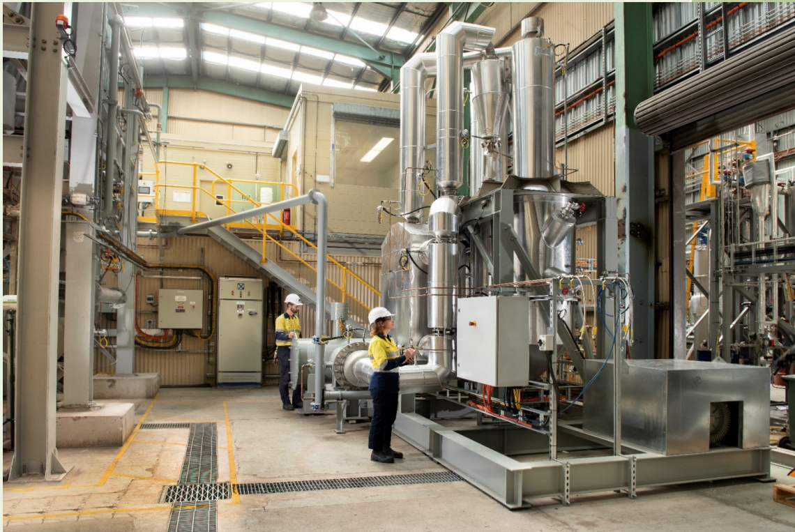
Photo of a pilot-scale version of UON's Regenerative Open Loop Calcium Cycle (ROL2C) which forms the basis of the PFAS Harvester technology.
