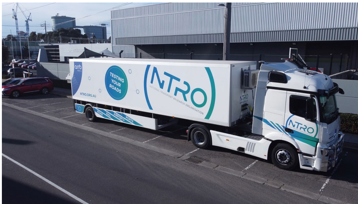
Figure 1 – Intelligent Pavement Assessment Vehicle (iPAVE)
