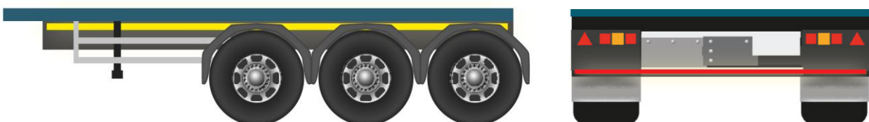
Figure 18: Semi-trailer with tray and line markings 6
