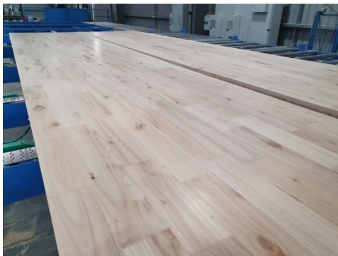
CLT manufactured in Tasmania by CLTP Tasmania Pty Ltd from E. nitens plantation hardwood
